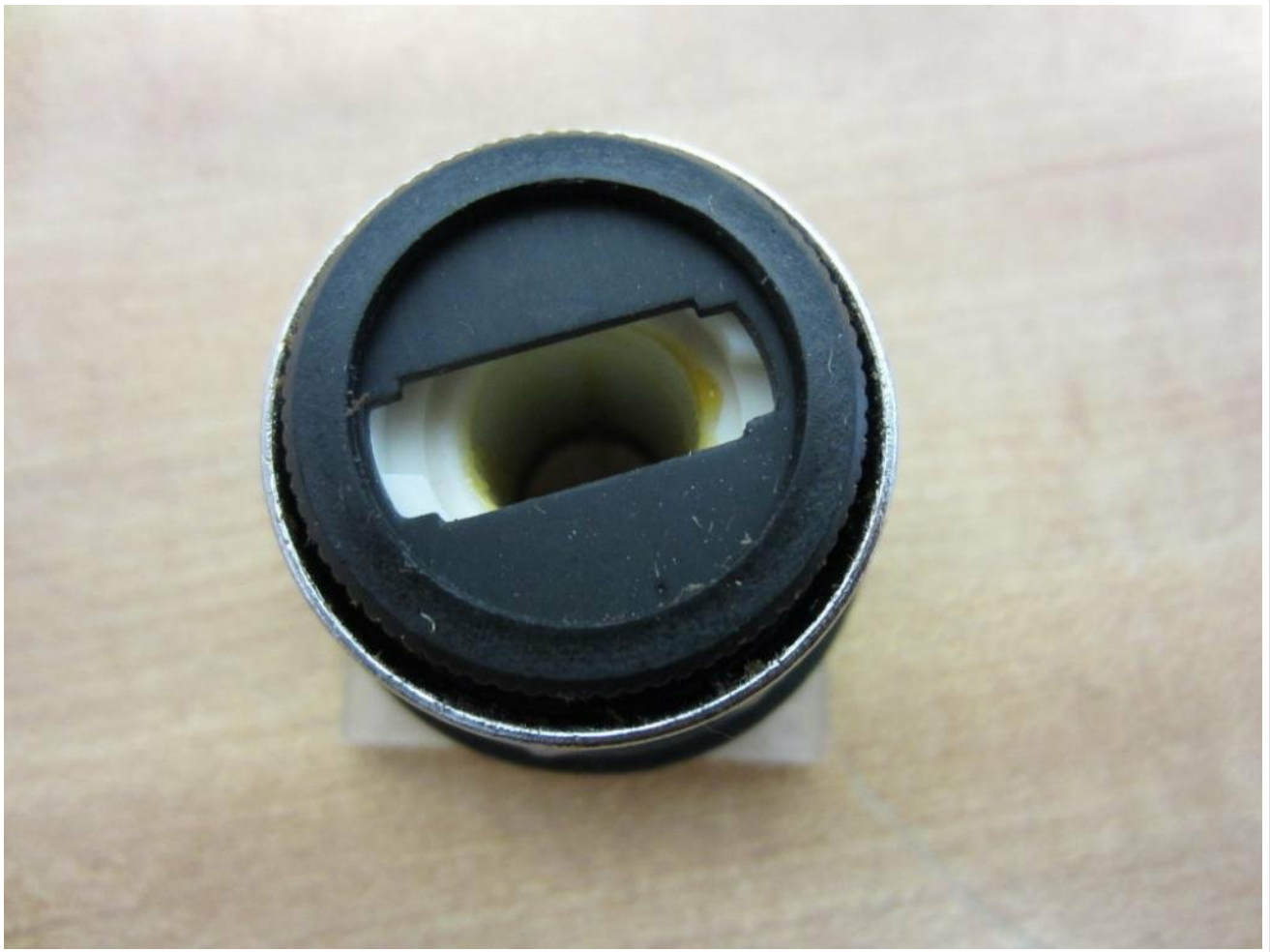
Figure 5: Top View of Actuator. This image provides a top-down view of the Square D 9001KS52 selector switch actuator, showing the slot for a key or lever, indicating its rotational capability.
