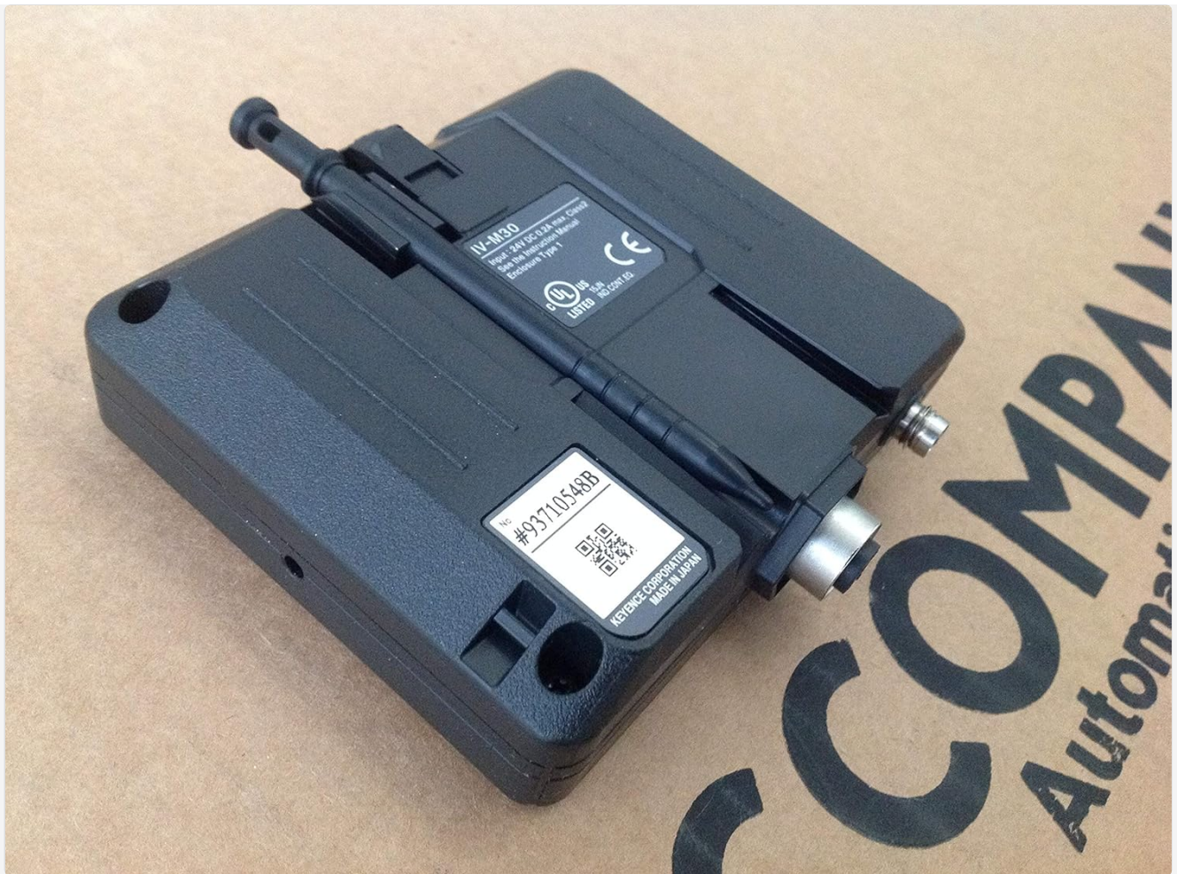
Figure 4: Rear view of the Keyence IV-M30 Intelligent Monitor, highlighting the connection ports and product labels including model number and power requirements.
