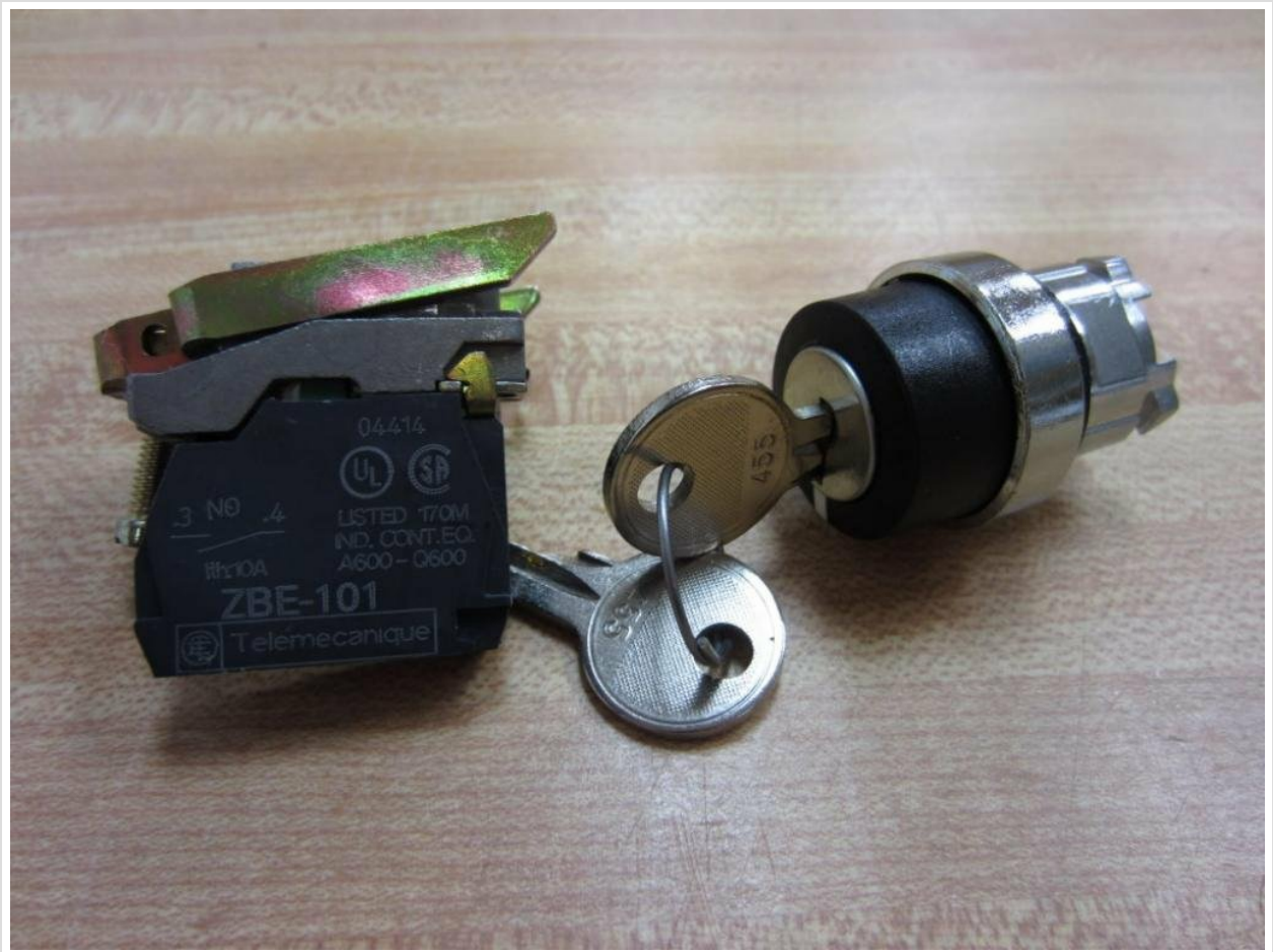
Close-up of the ZBE-101 contact block and one of the keys, highlighting the electrical ratings and Telemecanique branding.
