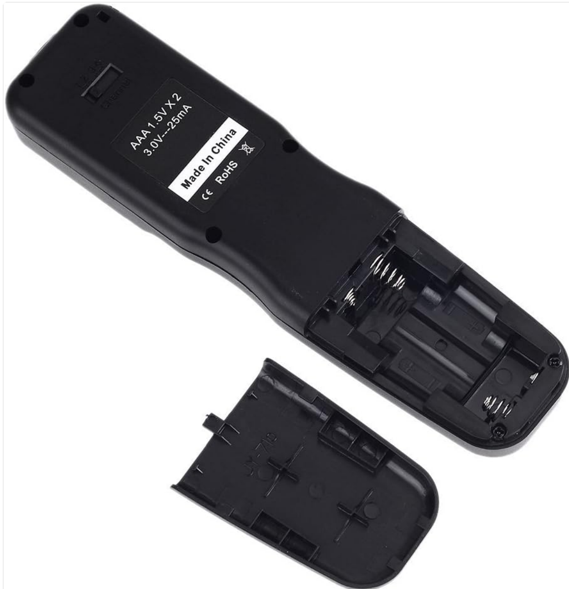
Figure 2: Rear view of the MC-C3 showing the battery compartment with the cover removed, ready for AAA battery insertion.
