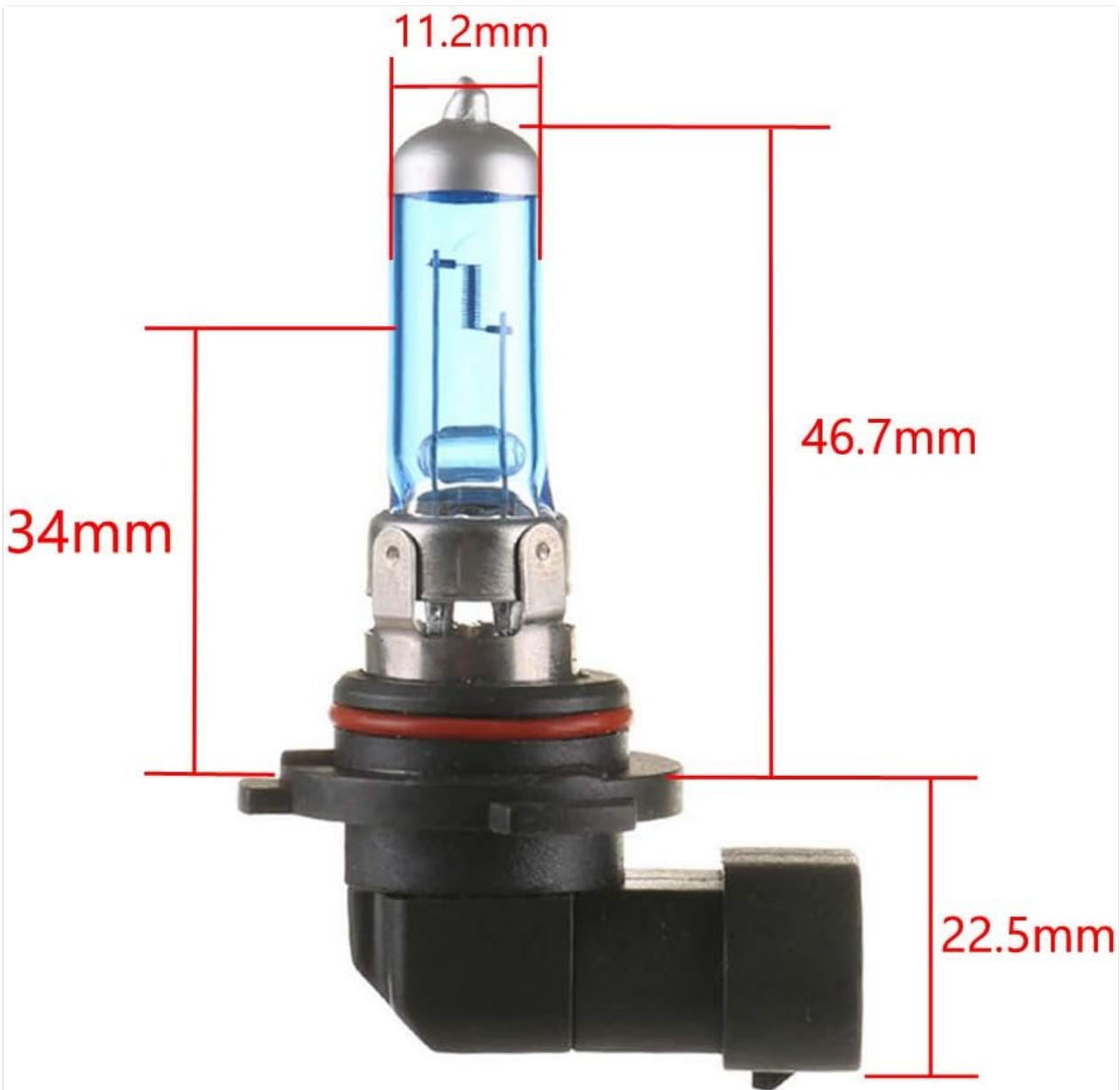
Image 7.1: Bulb base with specifications.
