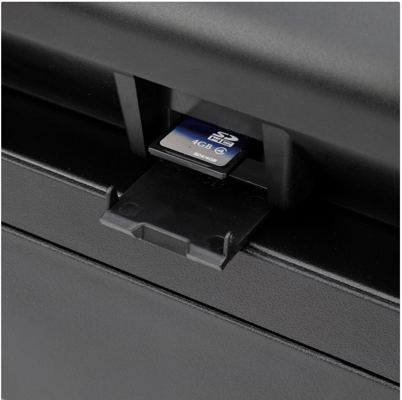
Figure 4.3.1: Detail of the SD card slot, used for transferring sales and programming data.
