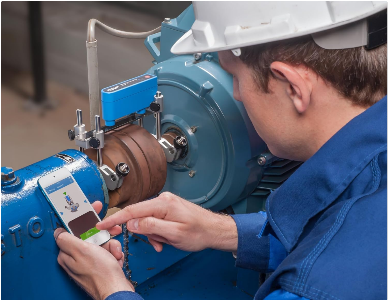
Figure 3: A technician interacting with the SKF TKSA 11 app on a smartphone while performing shaft alignment. The measuring unit is attached to the machinery in the background.
