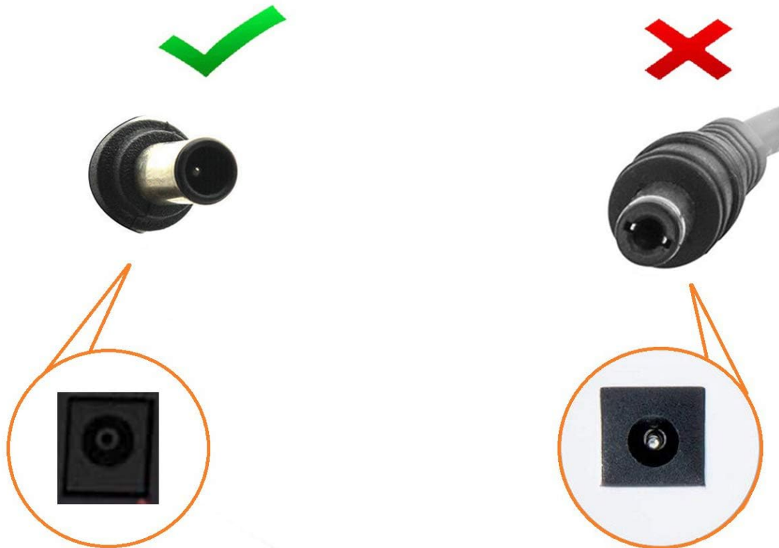
Figure 2: Illustration of compatible barrel connector (left) and incompatible connector (right). Ensure your device's port matches the compatible type.
