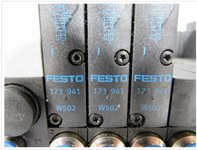
Figure 2: Detailed view of a valve module on the terminal, displaying the Festo brand and part number 173 941, along with a production code W502. This indicates specific component identification.
