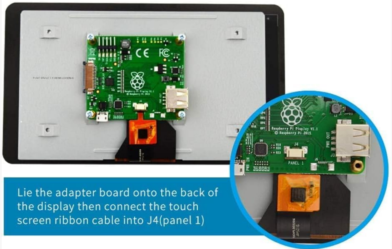
Figure 3.1: Connecting the adapter board and ribbon cable.
