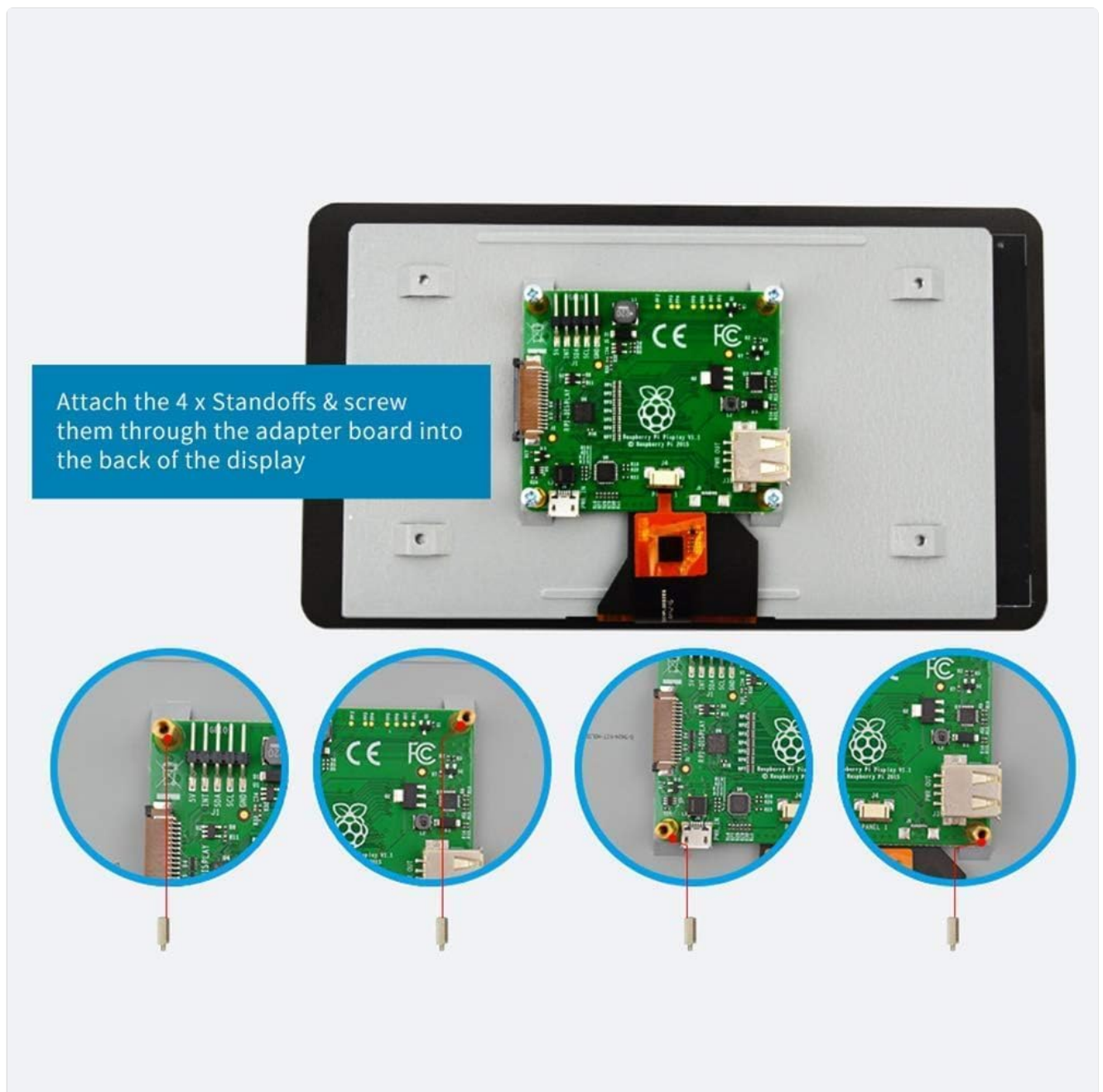
Figure 3.2: Attaching stand-offs and screws.
