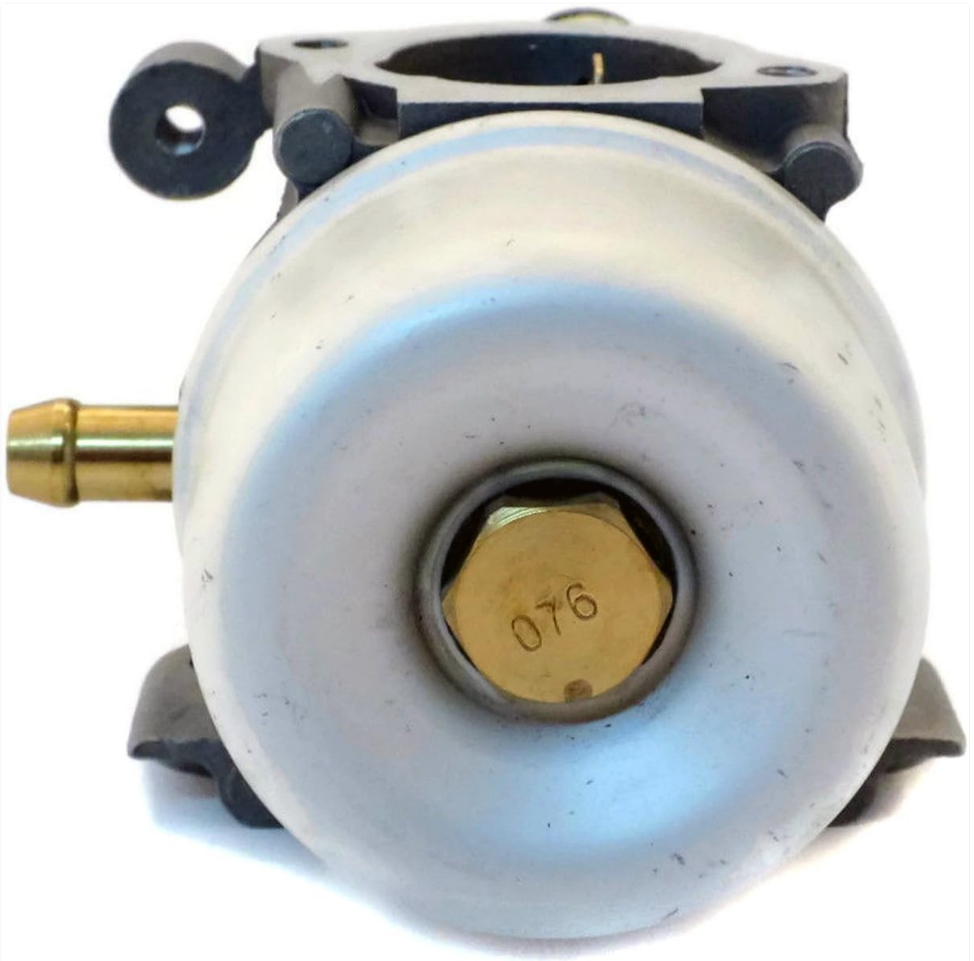
Figure 6.1: Bottom view of the carburetor, showing the float bowl. This section can be removed for cleaning if fuel contaminants are suspected.
