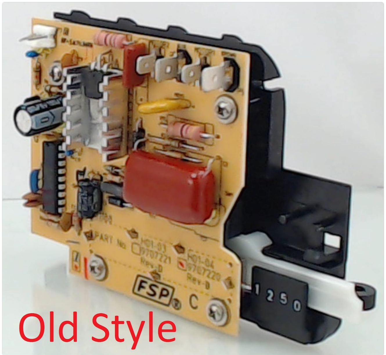
Figure 2: Close-up of an older style KitchenAid speed-control board, showing component layout and wiring points.
