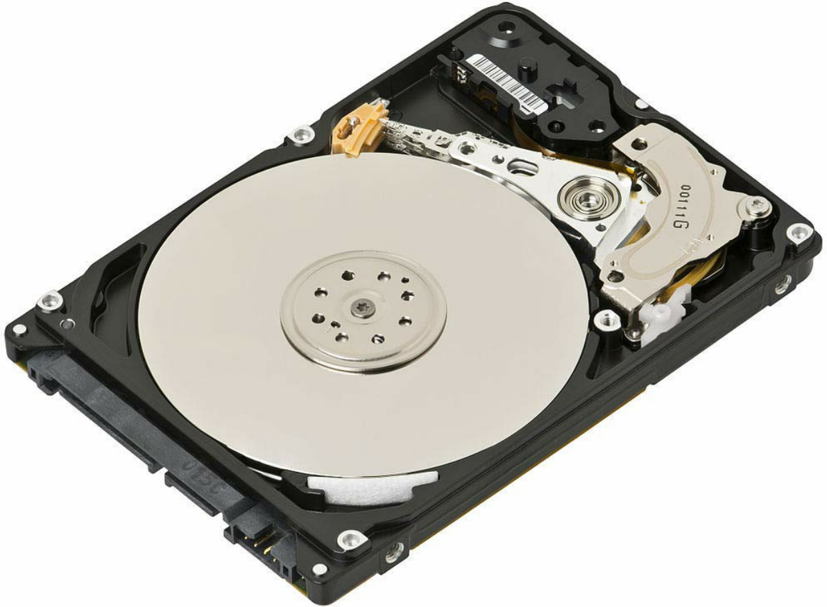
Figure 2.1: Internal view of the HP EG0600FBLSH 600GB SAS Hard Drive. This image displays the internal components of the hard drive, including the data platters and the read/write head assembly. The SAS data and power connectors are visible on the left side, indicating its interface type.
