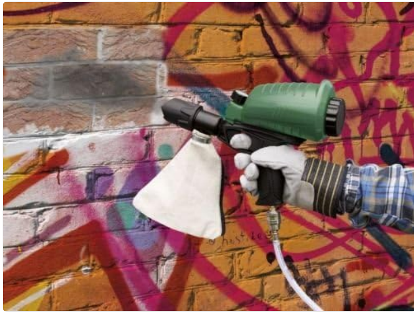
Image: The sandblasting gun being used on a brick wall to remove graffiti or old paint, showing its effectiveness on larger, textured surfaces.
