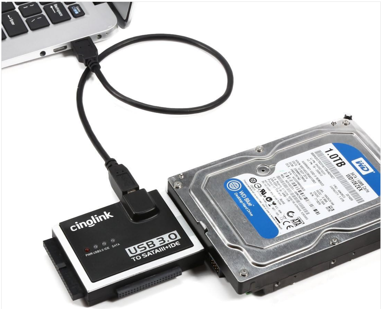
An image displaying the Cinglink SATA IDE to USB 3.0 Adapter, the USB 3.0 cable, the 12V 2A power adapter with an ON/OFF switch, and a 4-pin IDE power cable, alongside a connected 3.5-inch SATA hard drive.
