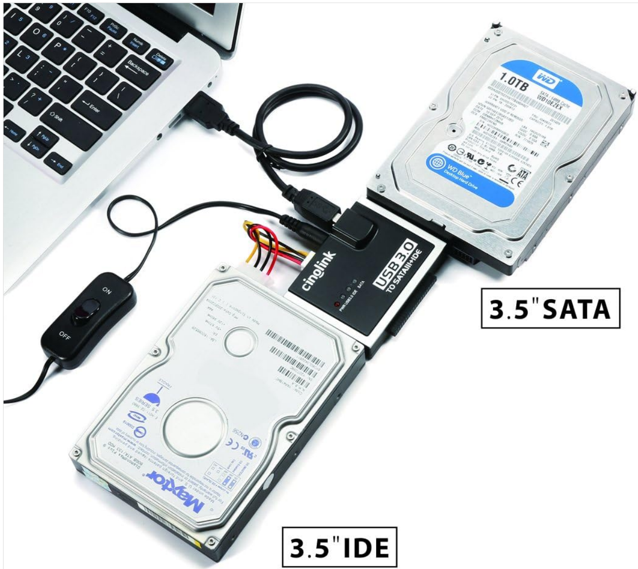
A 3.5-inch IDE hard drive connected to the Cinolink adapter, which is then connected to a laptop via USB. The power adapter and 4-pin IDE power cable are also shown connected.
