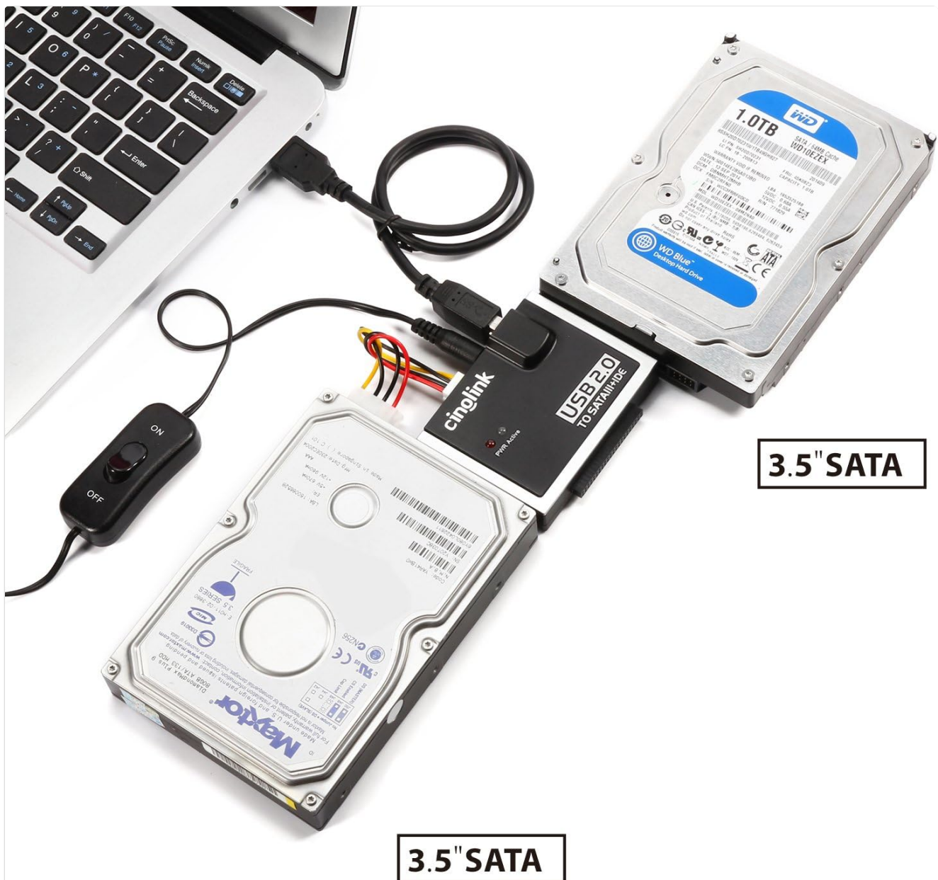
Figure 3.2: Connecting 3.5" SATA drives to the adapter and computer.
