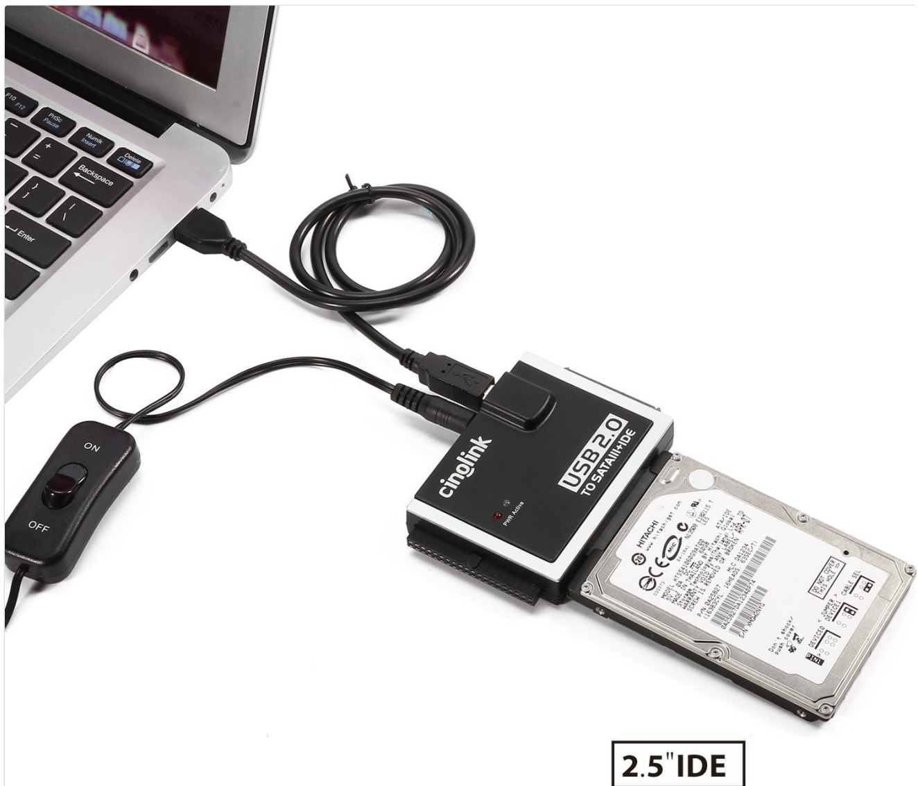
Figure 3.3: Connecting a 2.5" IDE drive to the adapter and computer.
