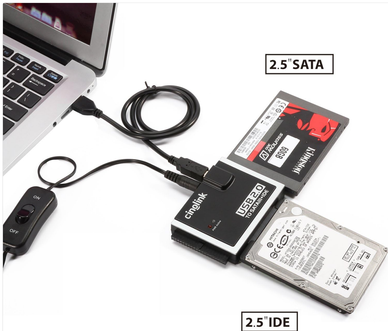
Figure 3.4: Simultaneous connection of 2.5" SATA and 2.5" IDE drives.
