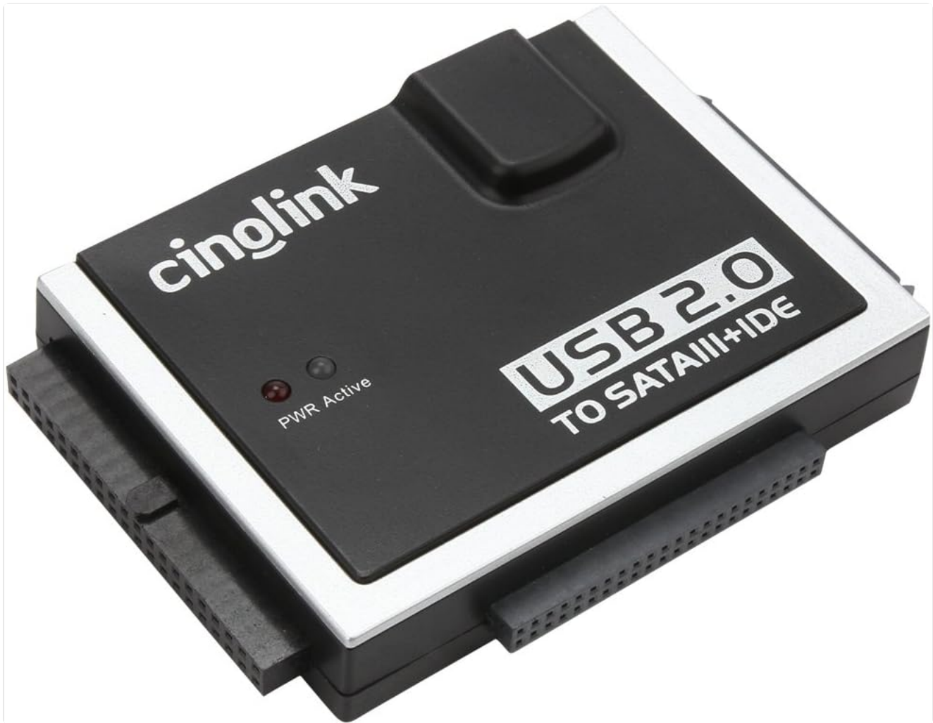
Figure 4.1: Close-up of the adapter with the "PWR Active" LED.
