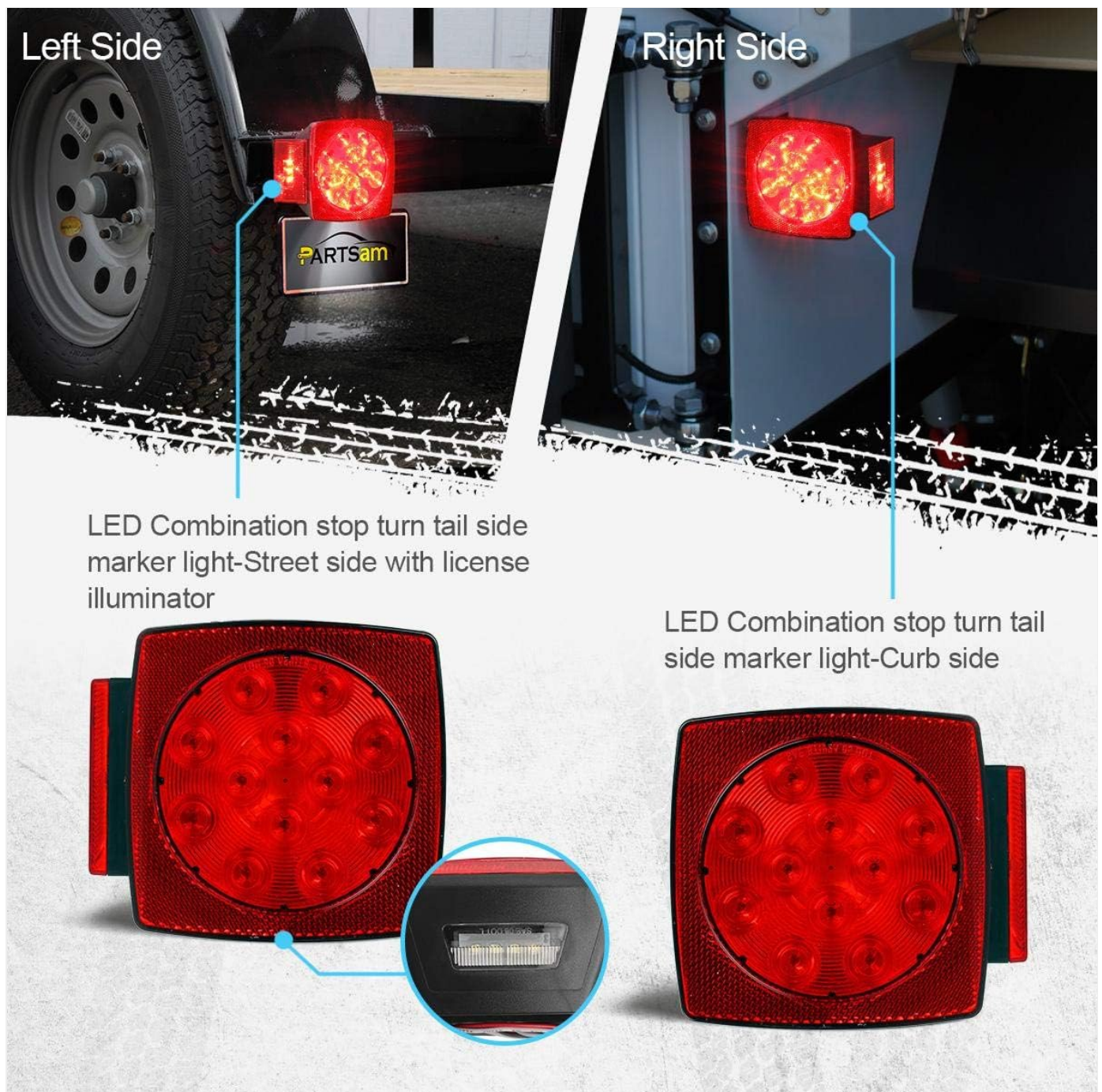
Figure 5.3: Visual representation of the left (driver) and right (passenger) side trailer lights, showing the integrated license plate illuminator on the driver's side.
