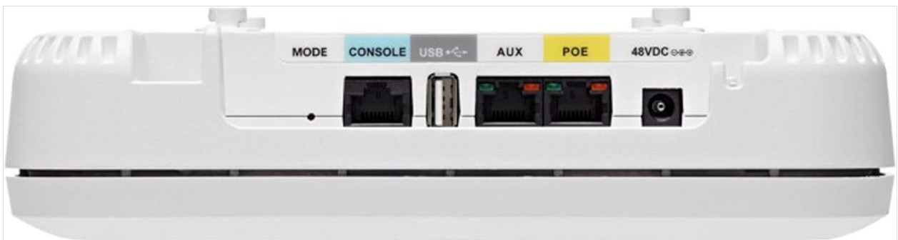
Figure 2: Rear view of the Cisco Aironet 1852I-B-K9 Wi-Fi Access Point, detailing the available ports. From left to right, these include a MODE button, CONSOLE port (RJ-45), USB-A port, AUX port, POE (Power over Ethernet) ports, and a 48VDC power input.
