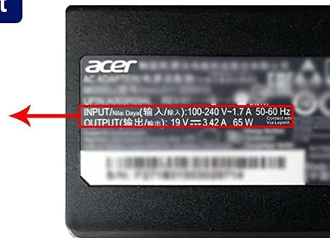
Image 4.2: Instructions for checking laptop and original adapter specifications for compatibility.
