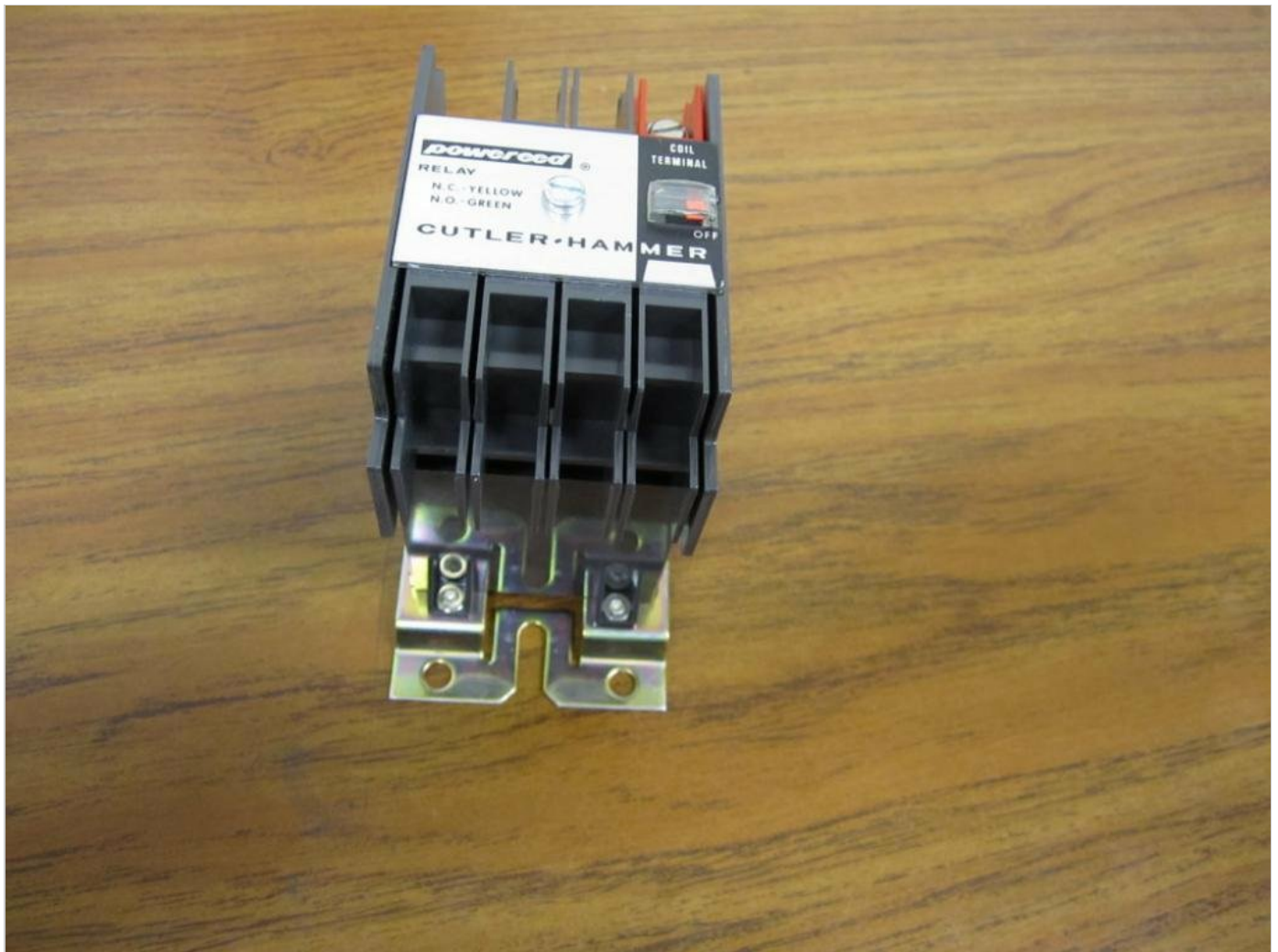
Image 3: Front view of the Cutler Hammer D40RB Powereed Relay, showing the "COIL TERMINAL" and "OFF" switch, along with labels for N.C. (Yellow) and N.O. (Green) poles.
