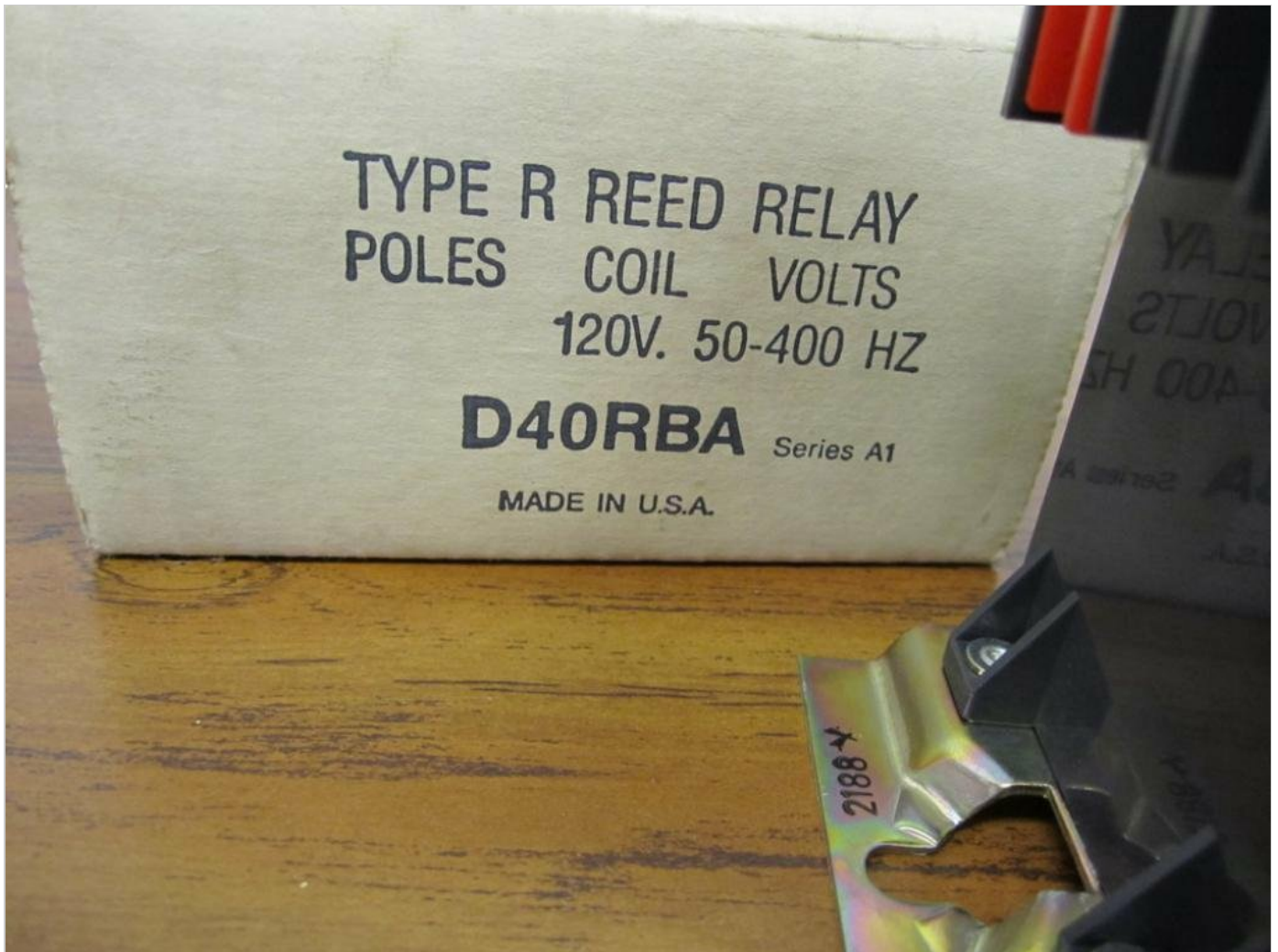
Image 2: A close-up view of the product box label, showing "TYPE R REED RELAY", "POLES COIL VOLTS 120V. 50-400 HZ", and "D40RBA Series A1". This confirms the coil specifications.
