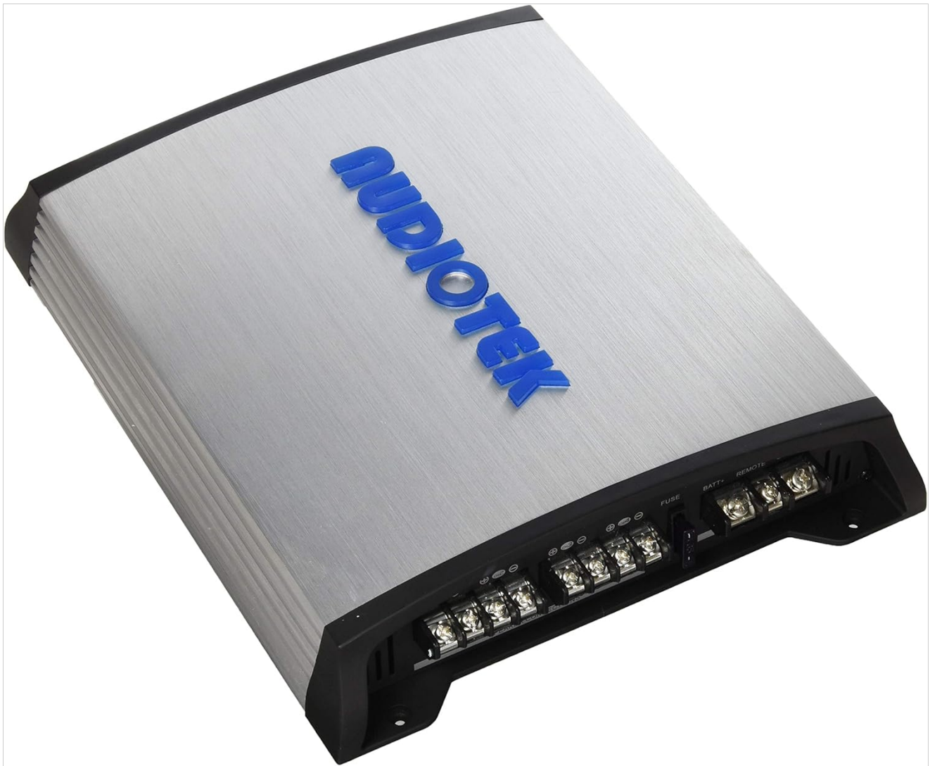
Image 1: Audiotek AT804S Amplifier showing power, ground, remote, and speaker output terminals. The fuse holder is also visible.
