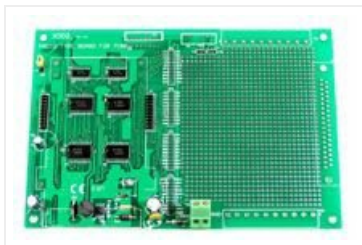
Figure 1: An overhead view of the ICP DAS X002 Prototype Board, showing its green PCB, integrated circuits, connectors, and a large prototyping area.
