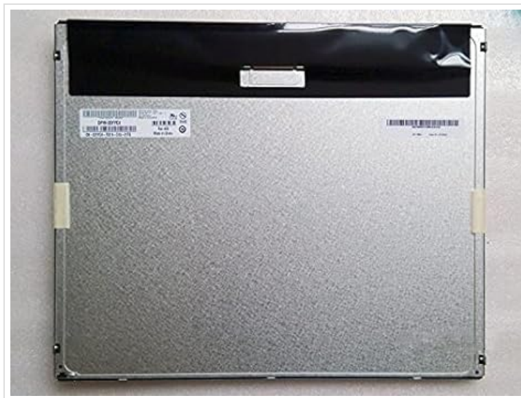
Figure 1: Rear view of the AUO M170ETN01.1 LCD Panel. This image displays the metallic back panel, which houses the internal components and connection interfaces. The top section is covered by a black protective material, and a label with product information is visible on the left side.
