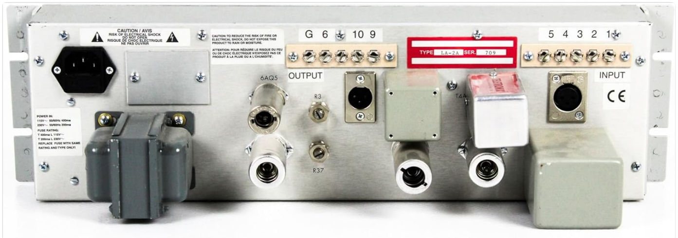
Figure 2: Rear panel of the LA-2A, illustrating the power input, audio input, and audio output connections.
