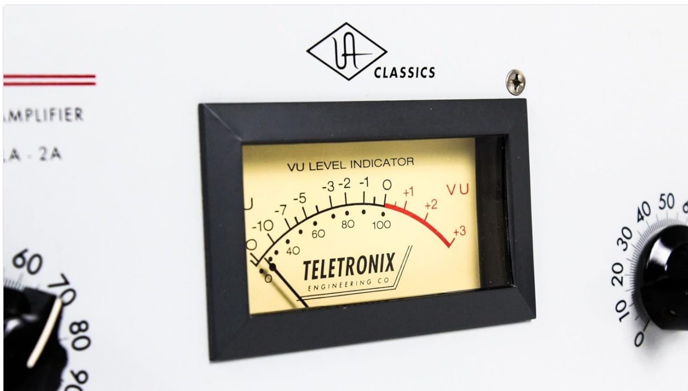
Figure 4: The illuminated VU meter, essential for monitoring gain reduction and output levels.
