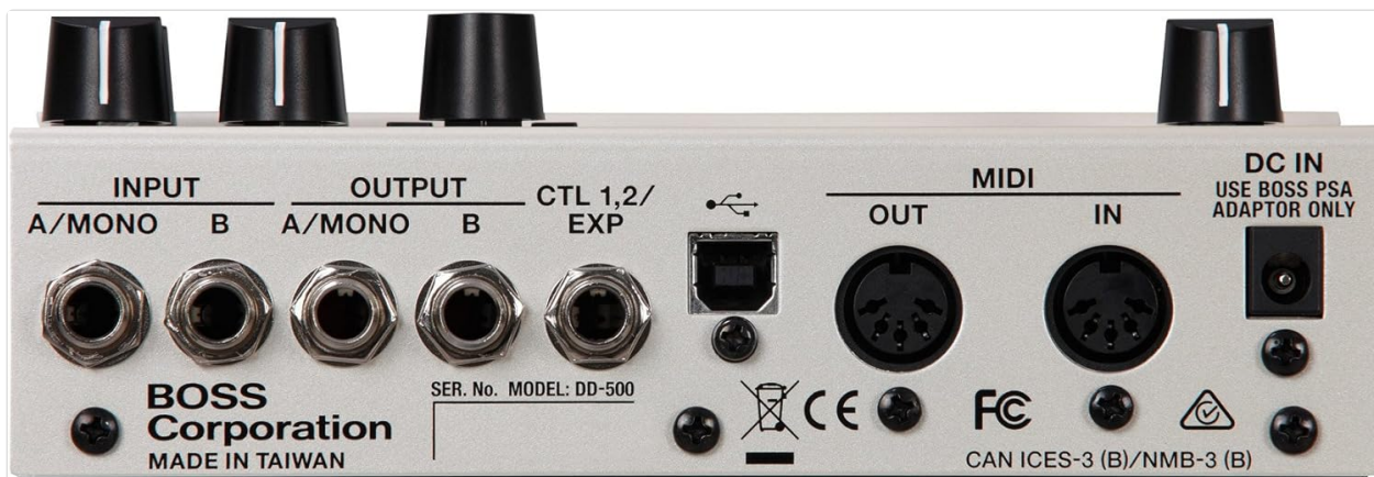
Figure 2: Rear panel of the DD-500, illustrating input, output, CTL/EXP, MIDI, and DC IN connections.
