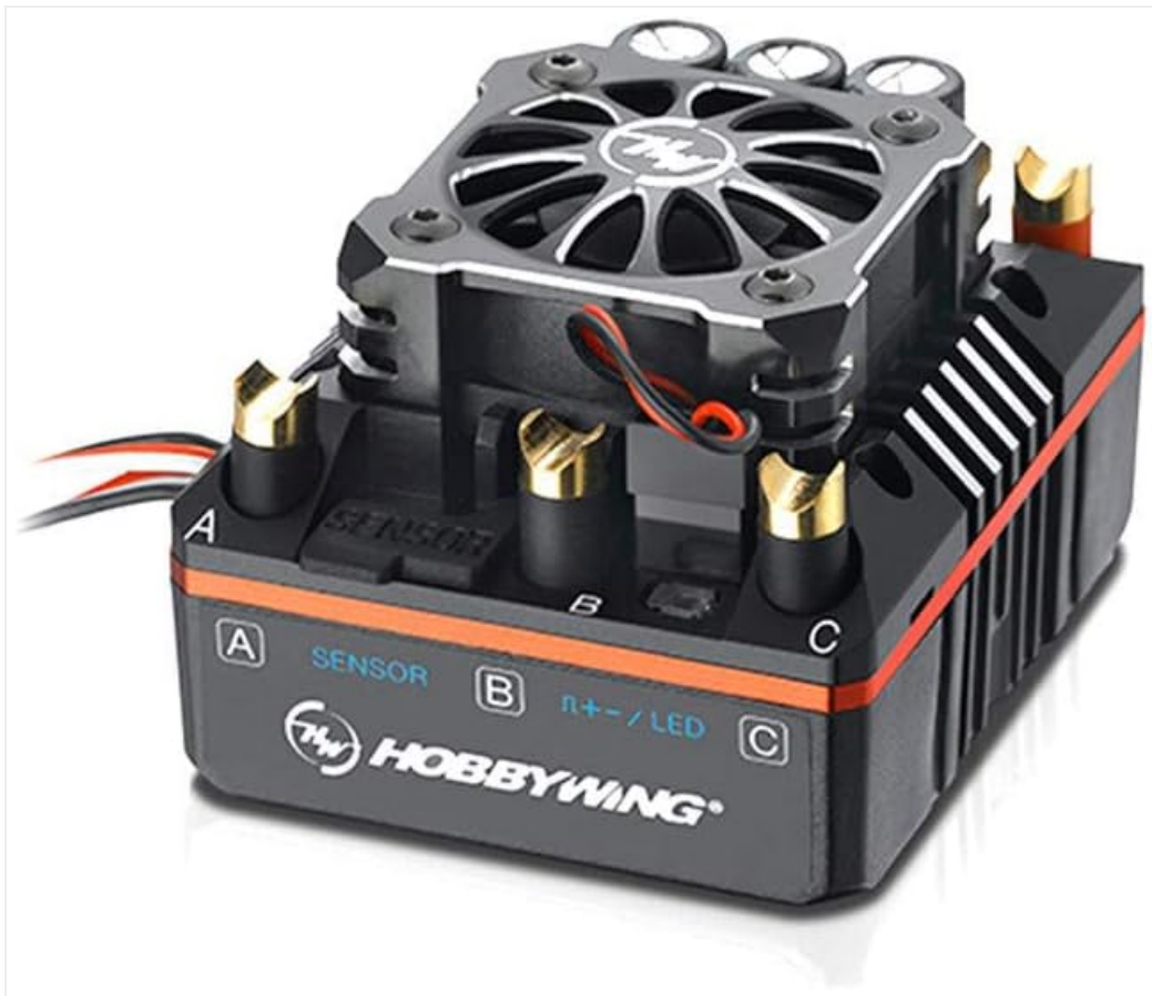
Figure 1: Top view of the Hobbywing XeRun XR8 Plus Speed Controller, showing the cooling fan, capacitor bank, and motor output terminals (A, B, C) along with the sensor port.
