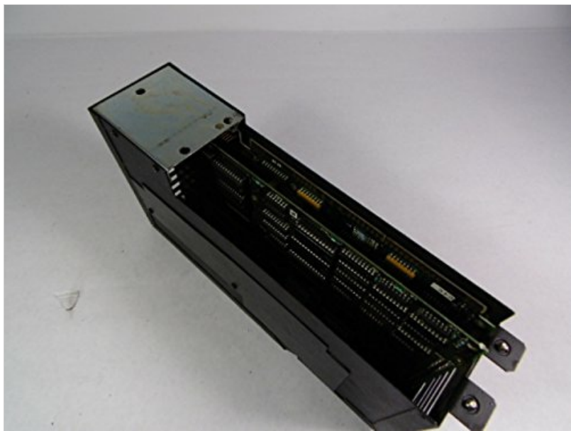
Figure 3.2: Side view of the Square D 8020-SCP-522 Processor Module, revealing the internal circuit boards and connectors.
