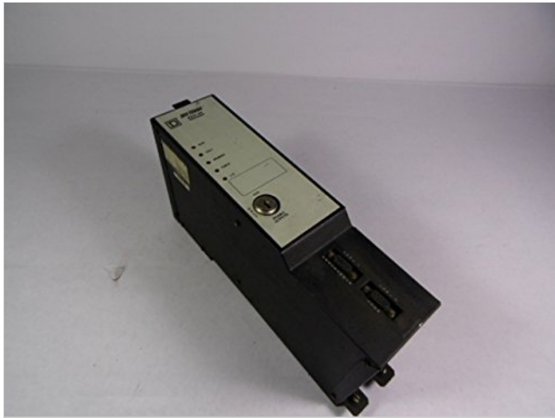
Figure 3.1: Front view of the Square D 8020-SCP-522 Processor Module, showing the status indicators and key lock.
