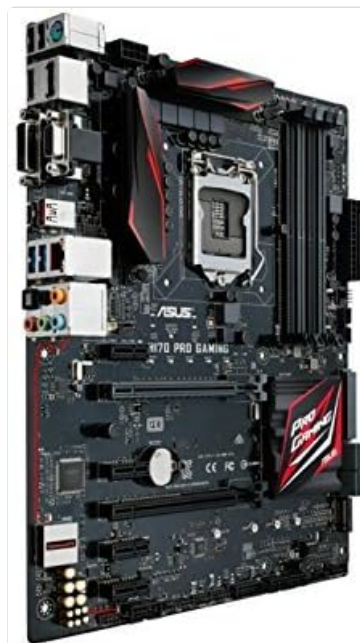
Figure 2.2.2: Angled view of the ASUS H170 PRO GAMING Motherboard, highlighting the I/O ports and the overall layout within a system.
