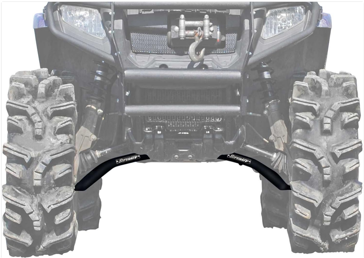
A pair of black SuperATV High Clearance 1.5 inch Forward Offset A-Arms, designed for Polaris Sportsman models. These arms are built from robust alloy steel.
