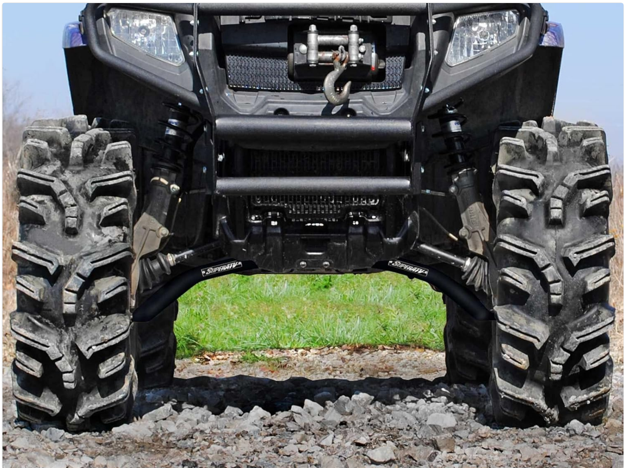
Front view of a Polaris Sportsman ATV equipped with SuperATV High Clearance A-Arms, demonstrating the enhanced ground clearance and space for larger tires.
