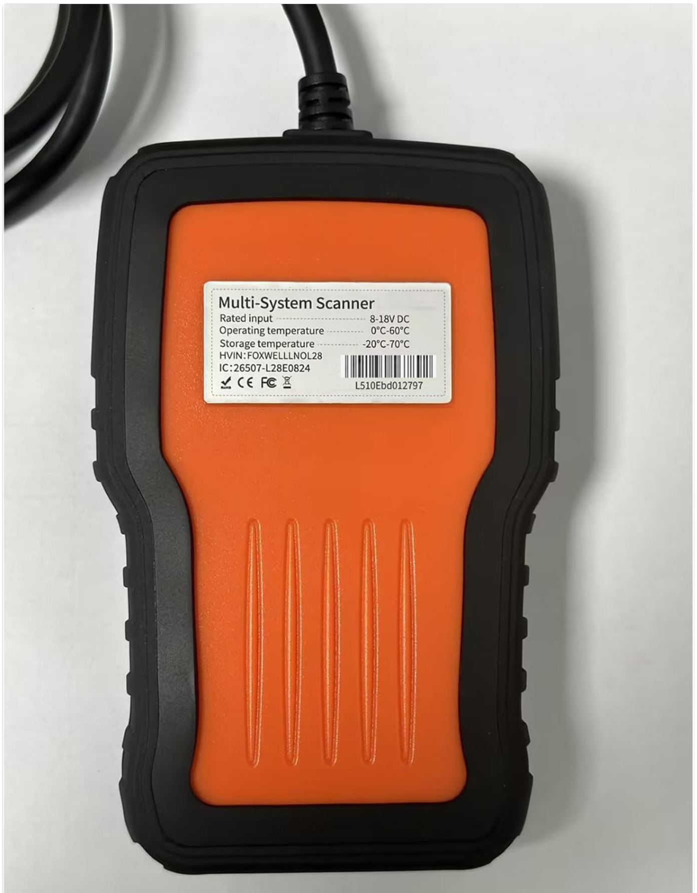
Figure 7.1: Product label on the back of the NT510 Elite, detailing input voltage, operating temperature, and storage temperature.
