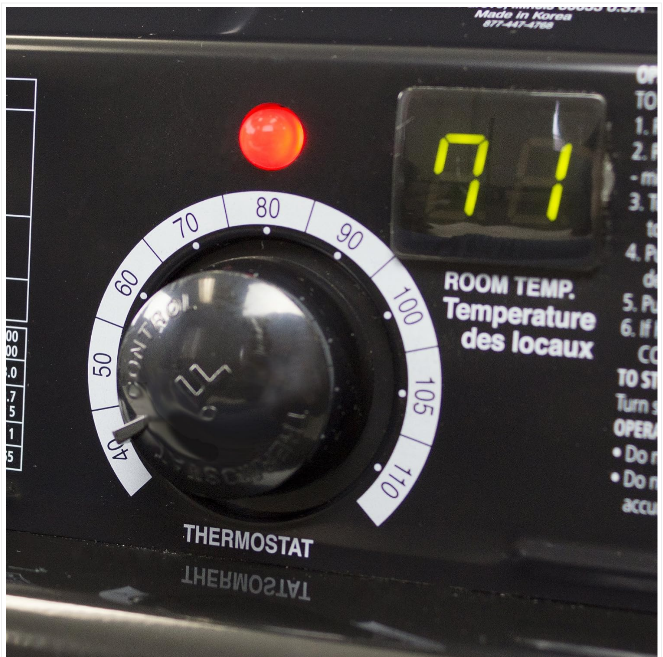
Figure 8: Digital thermostat control. The dial allows precise temperature adjustment, and the LED screen displays the current setting.
