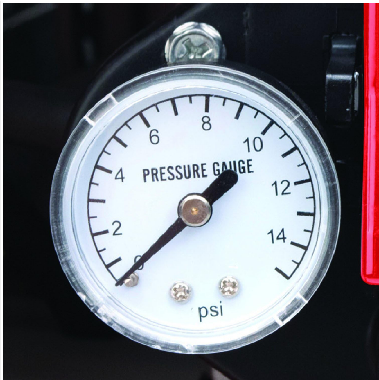
Figure 9: Close-up of the air pressure gauge. This gauge helps ensure the heater is operating within safe and efficient pressure ranges.
