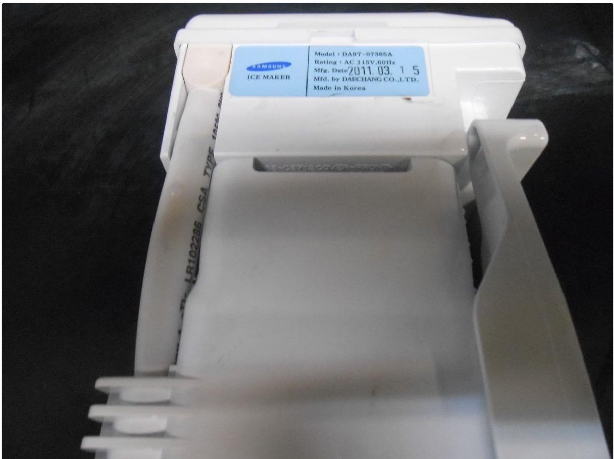
Figure 2: Close-up view of the ice maker's identification label. The label clearly indicates "Model: DA97-07365A", "Rating: AC 115V 60Hz", and "Mfg. Date: 2011.03.15".
