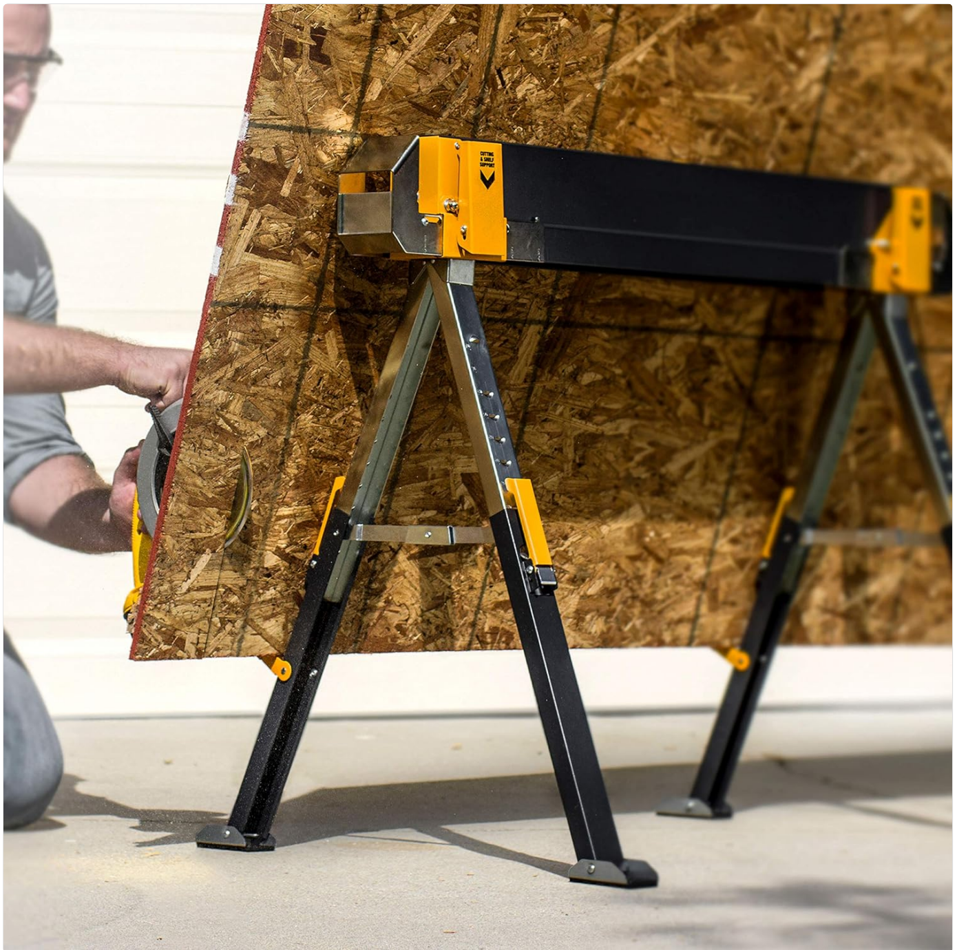
Figure 5: Using the side support pegs for vertical material cutting.
