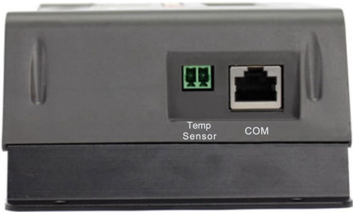
Figure 3: Side Panel. This image illustrates the side of the controller, featuring the dedicated ports for the external temperature sensor and the COM (communication) interface, typically an RJ45 port for remote monitoring or PC connection.
