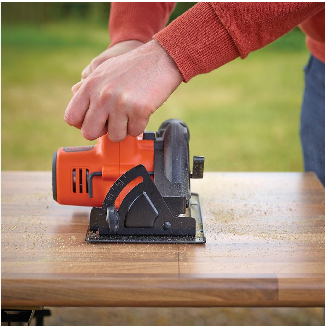
Figure 5: A close-up view of the circular saw's blade engaging with a wooden surface during a cut. Sawdust is being ejected, and the base plate is resting on the material.
