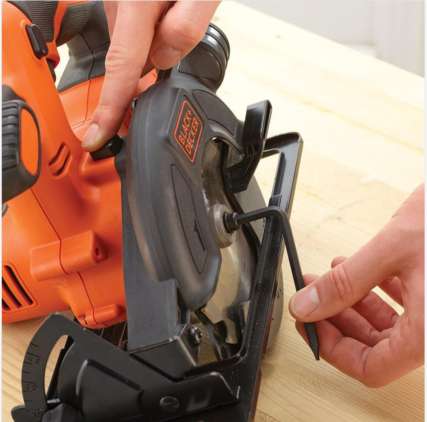
Figure 3: A user demonstrating the process of installing a new saw blade. The image shows a hand holding a hex key to loosen the blade clamp bolt, with the spindle lock button pressed.
