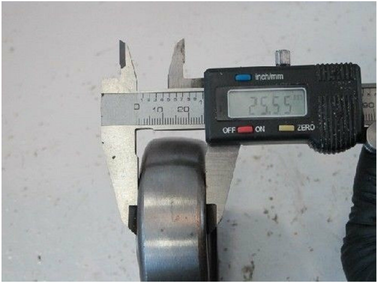
This image shows a digital caliper measuring the thickness or width of the Webb 15911 Unground Ball Bearing. The measurement displayed on the caliper is 25.55 mm.
