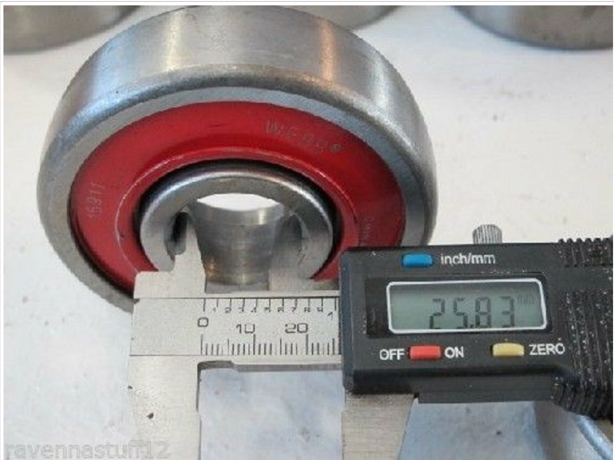
A digital caliper is used to measure the inner diameter (bore) of the Webb 15911 Uground Ball Bearing. The digital readout
