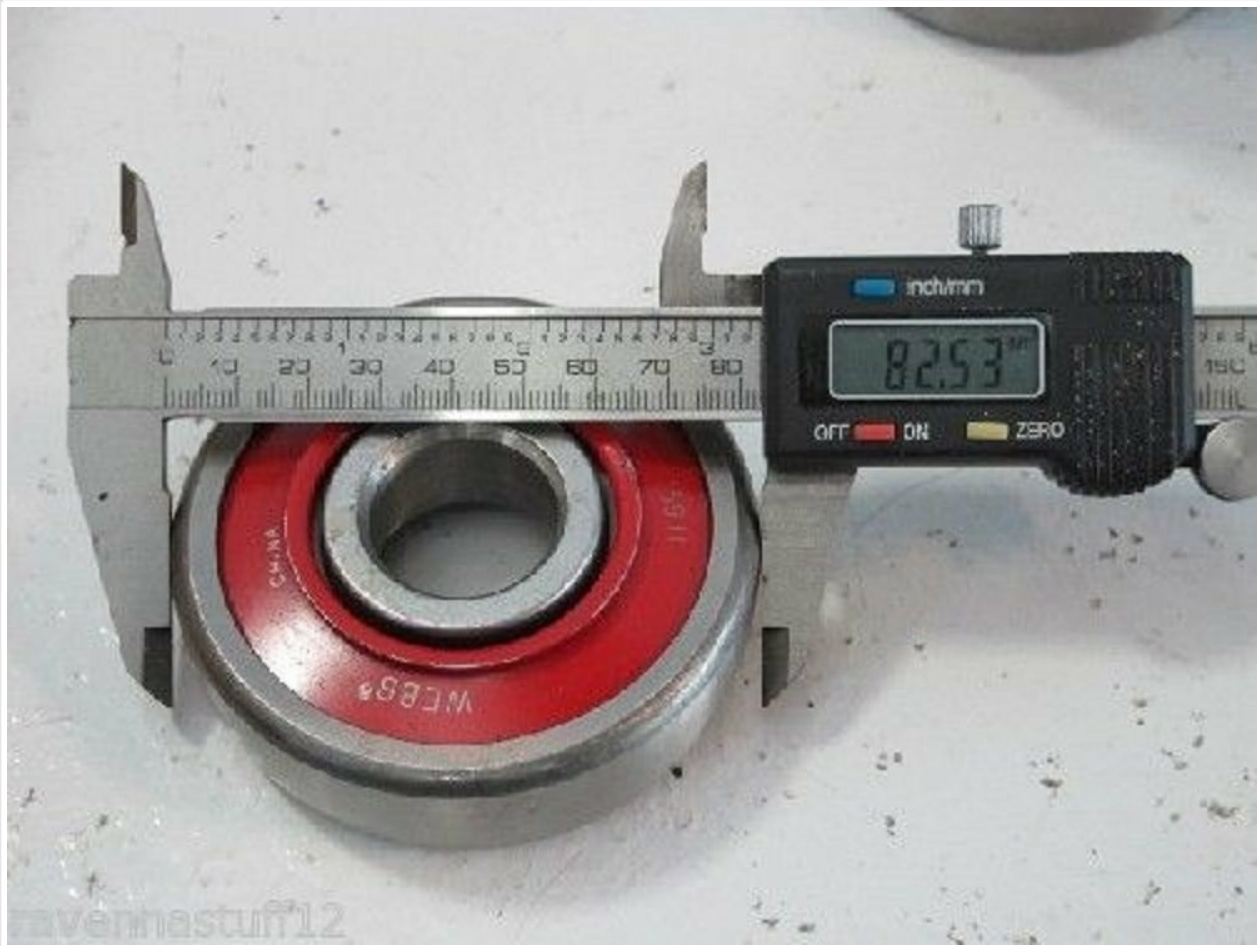
A digital caliper is shown measuring the outer diameter of the Webb 15911 Uground Ball Bearing. The display reads 82.53 mm, indicating the overall width of the bearing.
