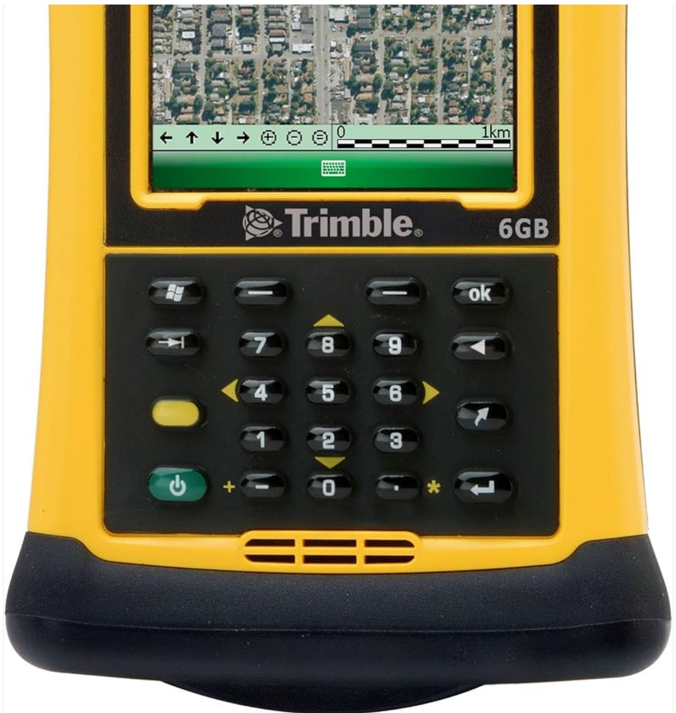
Figure 1: Front view of the Trimble Nomad 900LE handheld computer. The device is yellow and black, featuring a color display showing a topographic map, and a numeric keypad below it. The screen displays "NOMAD" at the top, "TerraSync" application, and "Trimble" logo at the bottom. The keypad includes numeric keys, navigation arrows, and function buttons.
