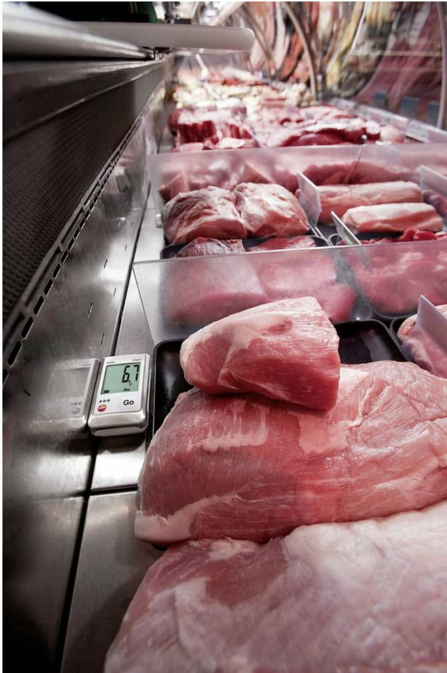
Figure 2: The Testo 175 T3 in use within a meat display case, demonstrating its application in food temperature monitoring.
