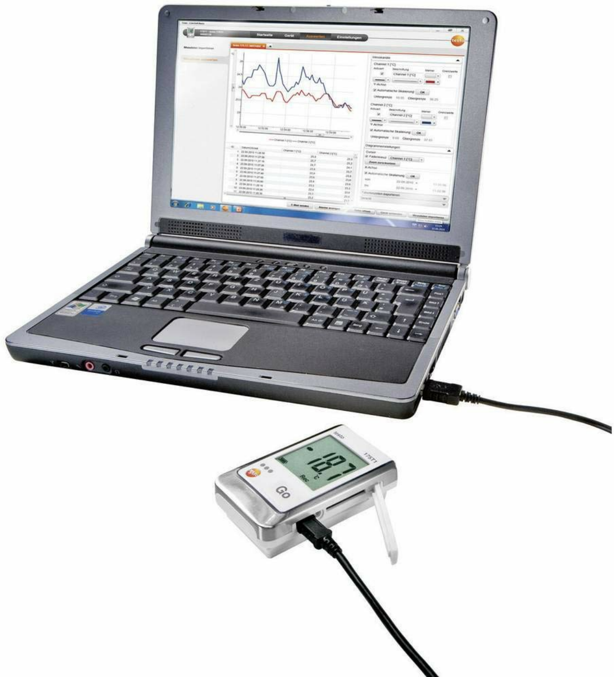
Figure 4: The Testo 175 T3 connected to a laptop for programming and data analysis using ComSoft software.
