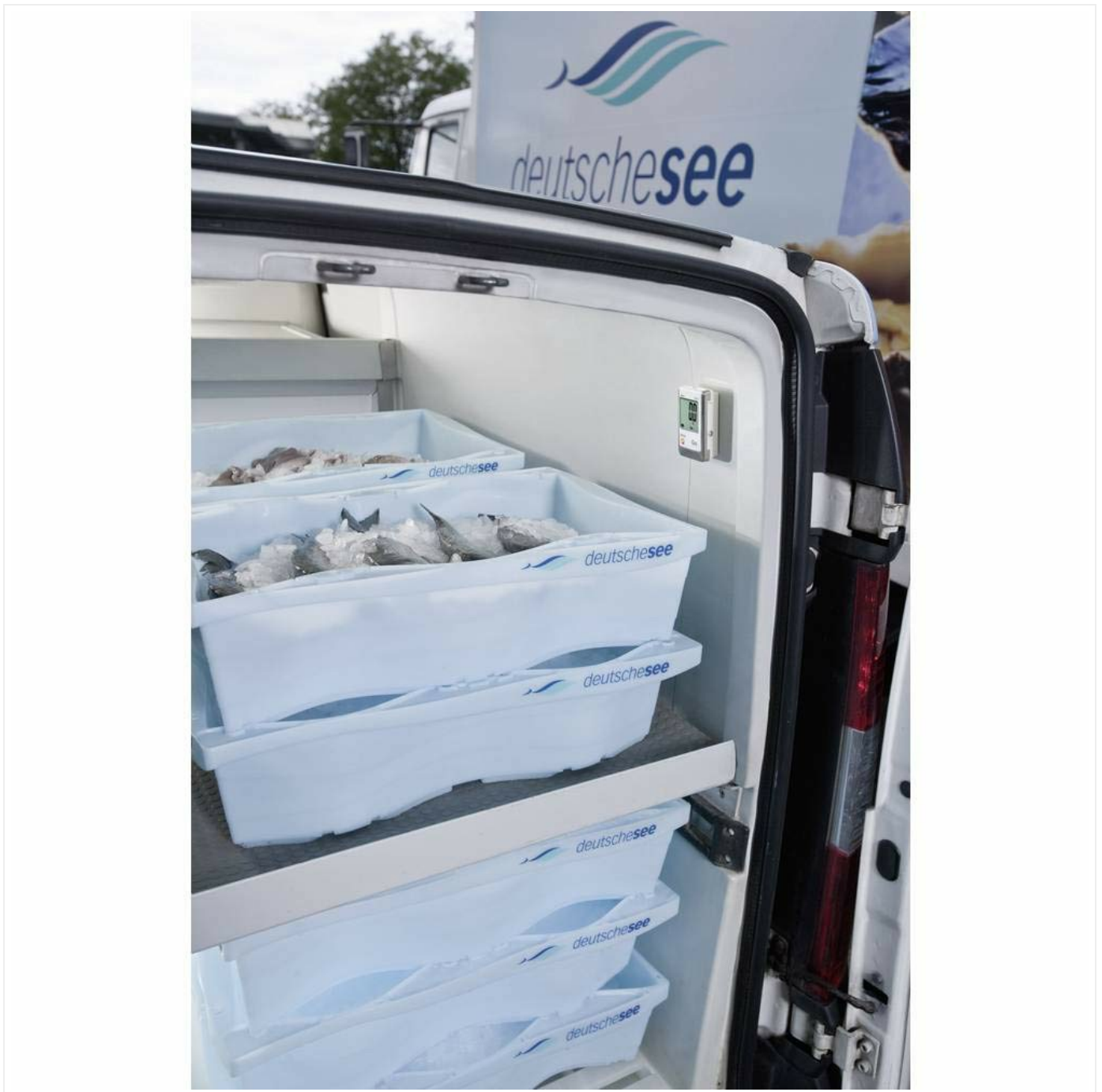
Figure 3: The Testo 175 T3 mounted inside a refrigerated transport vehicle, illustrating its use for monitoring temperatures during transit.
