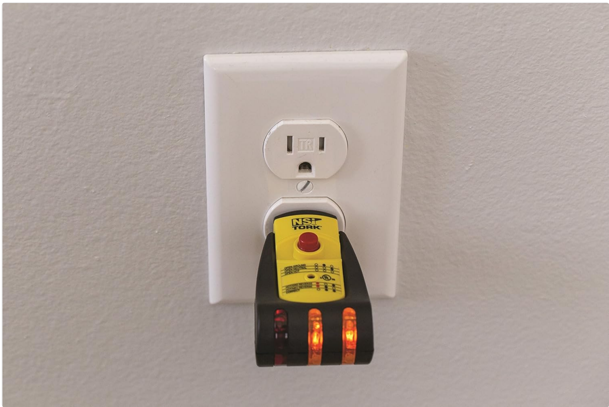
Figure 5: Close-up view of the TES-131's red push-button for initiating the GFCI integrity test.
