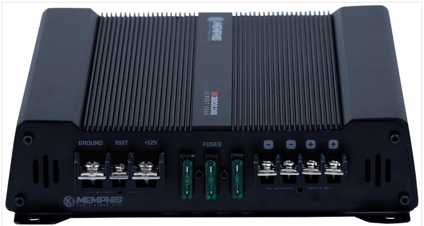
Image showing the power, ground, remote, and fuse terminals on the Memphis Audio SE3200.1V2 amplifier.
