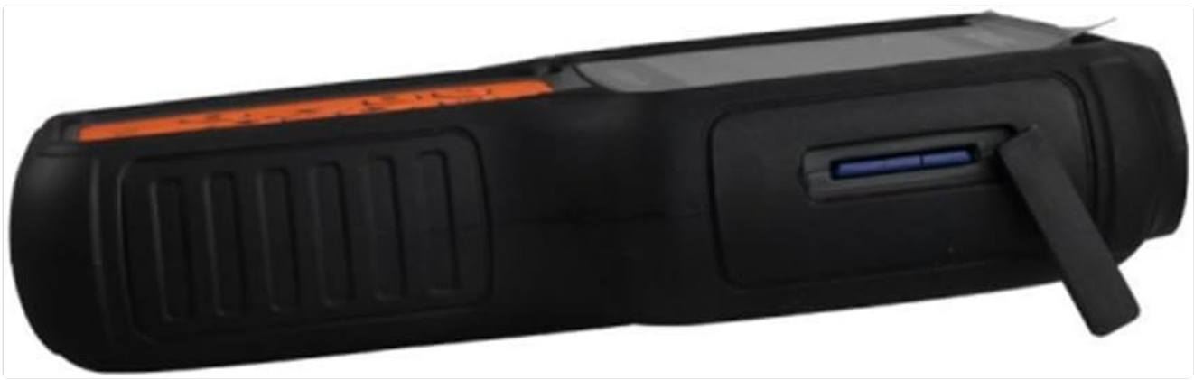
Figure 2.3: Side view of the scanner, highlighting the SD card slot and kickstand.
