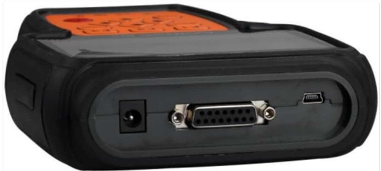
Figure 2.4: Bottom view of the scanner, showing the diagnostic port and USB port for connections.
