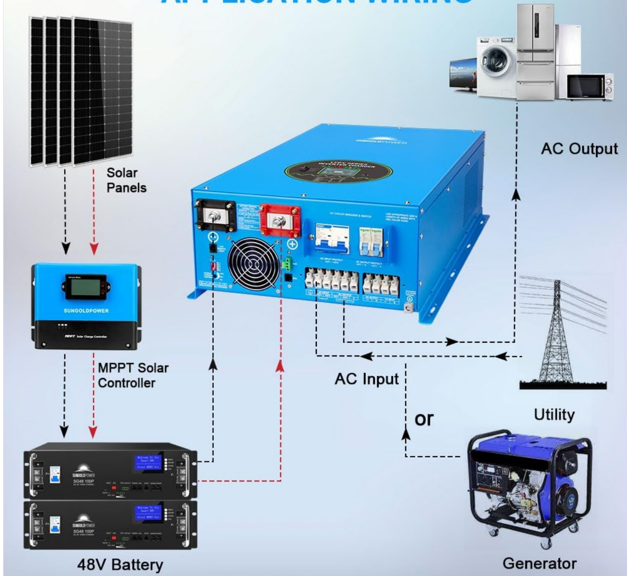
Figure 5.1: Typical application wiring diagram.
