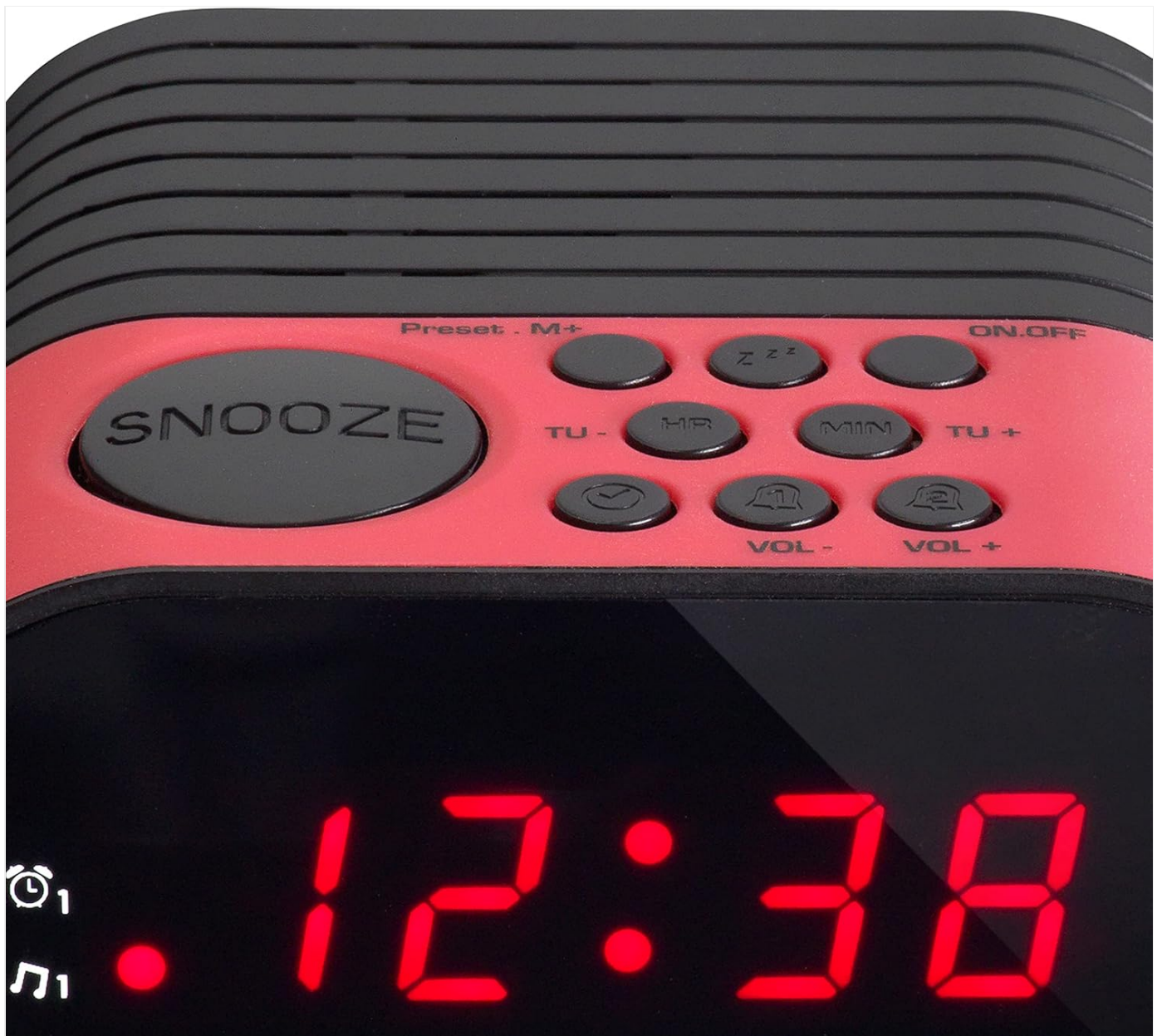
Figure 2: Close-up view of the control panel. Buttons visible include a large "SNOOZE" button, "ON.OFF", "Preset: M+", "TU-", "HR", "MIN", "TU+", "VOL-", and "VOL+". These buttons are used for setting time, alarms, tuning the radio, and adjusting volume.
