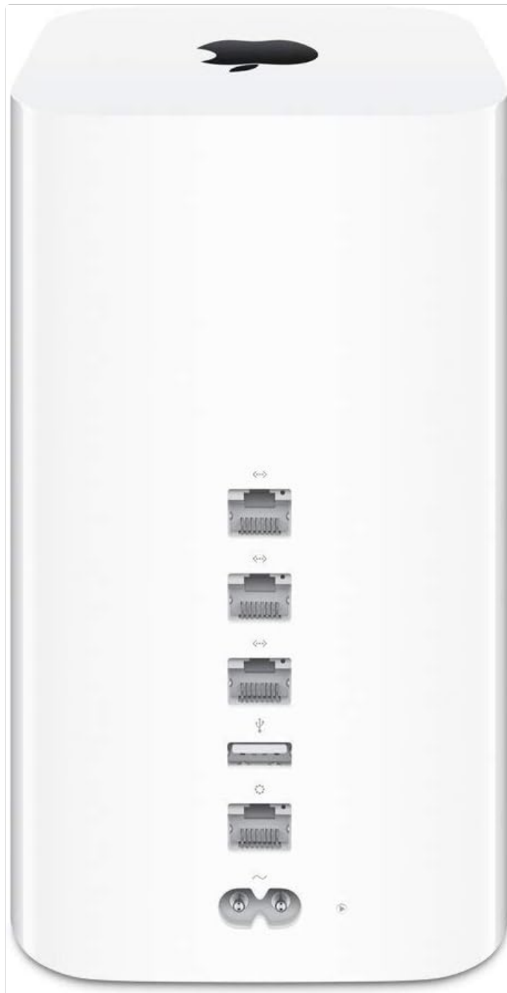
Figure 2: Rear view of the Apple AirPort Extreme Base Station, showing the various ports. From top to bottom, these include three LAN ports, a USB port, a WAN port, and the power input.
