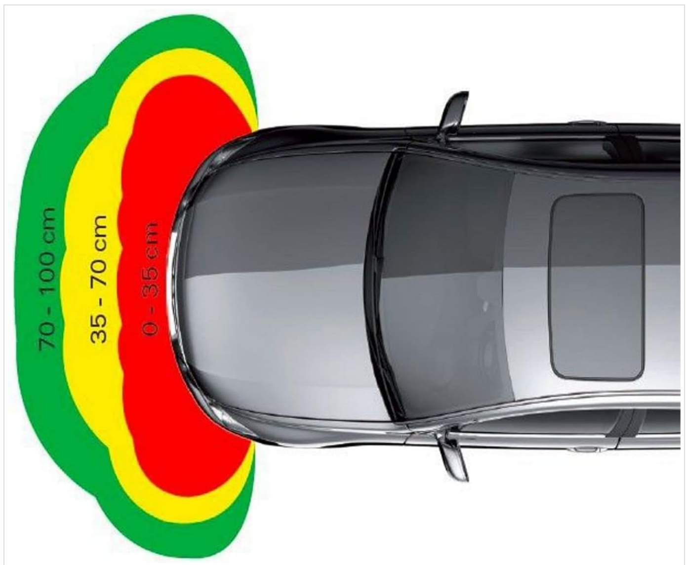
Figure 1: Illustration of the detection zones for the front parking aid system. The zones indicate varying distances where obstacles are detected, typically ranging from 0-35 cm (red), 35-70 cm (yellow), and 70-100 cm (green).
