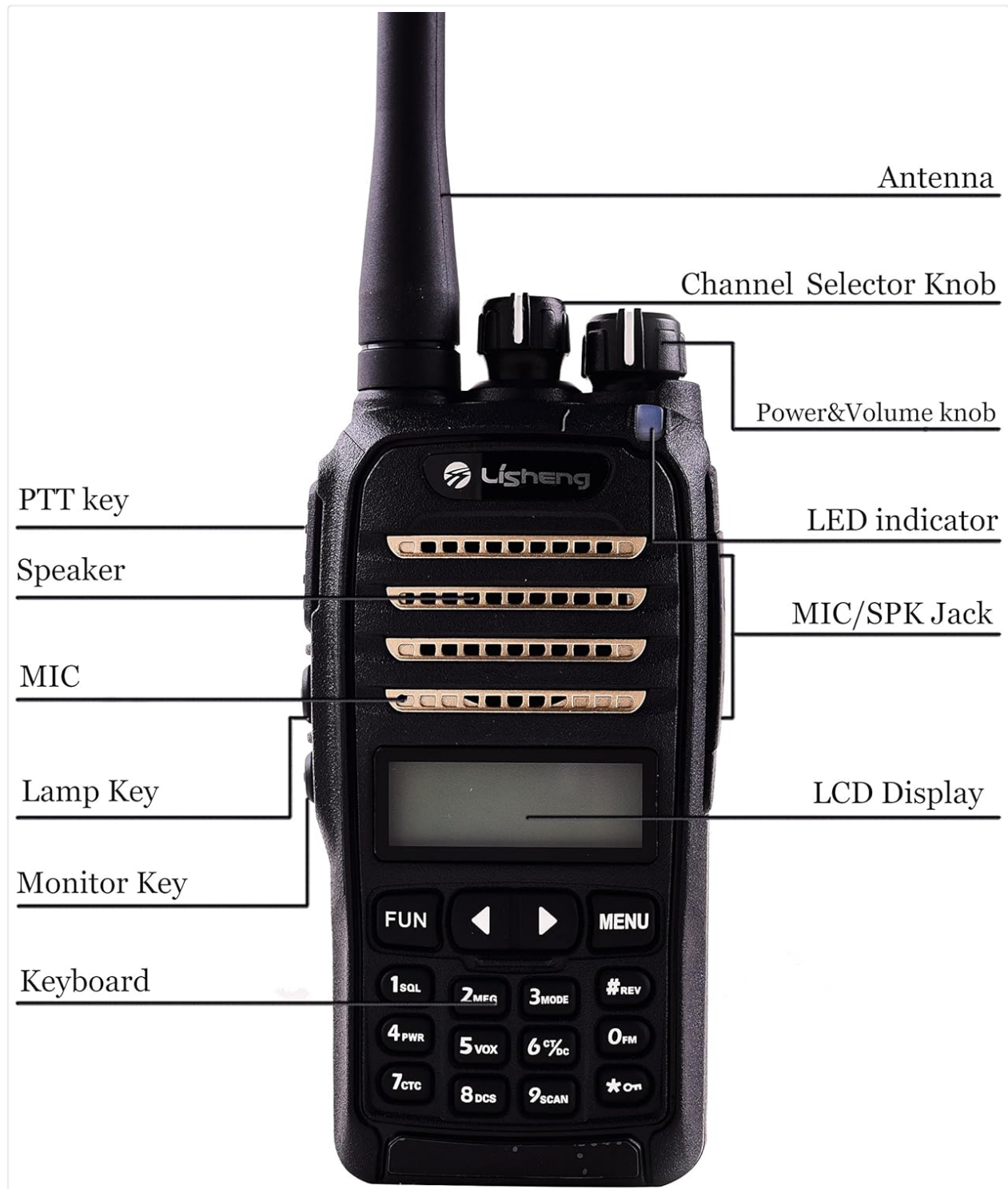
Figure 3.1: Front view of the LISHENG LS-747 radio with key components labeled. Labels include Antenna, Channel Selector Knob, Power&Volume Knob, LED indicator, PTT key, Speaker, MIC, MIC/SPK Jack, Lamp Key, LCD Display, Monitor Key, and Keyboard.
