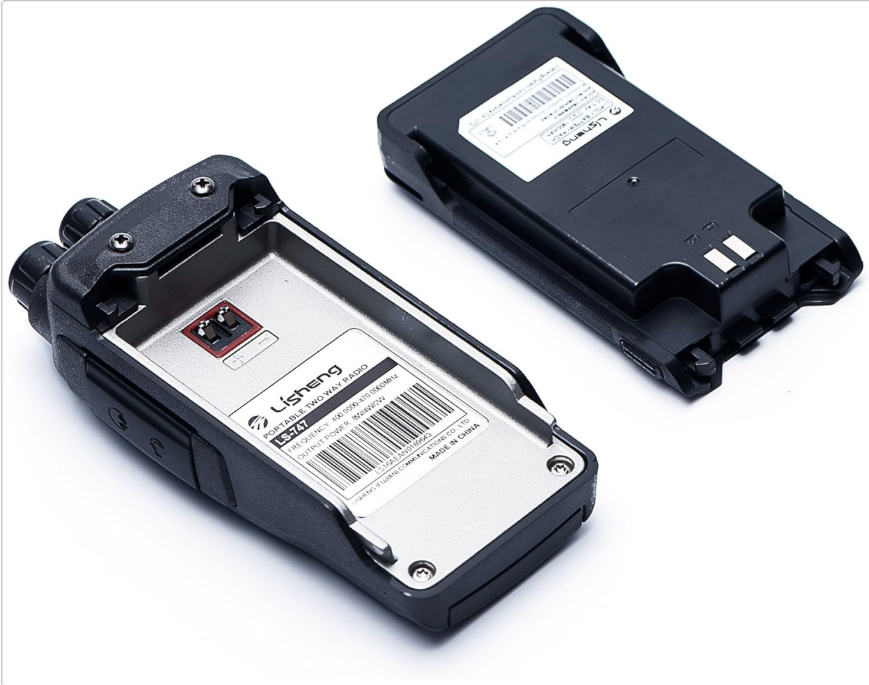
Figure 4.2: The LISHENG LS-747 radio with its battery compartment exposed and the battery pack shown separately, ready for installation or removal.
