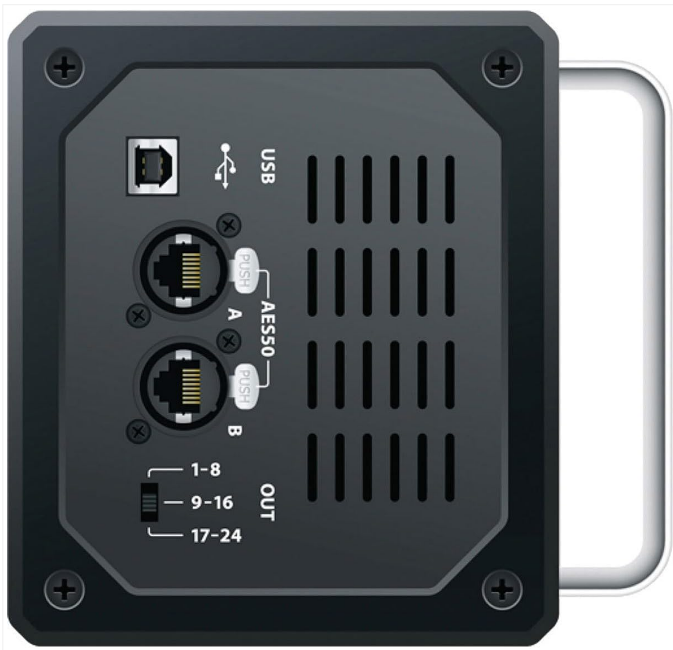
Figure 4: Left side view of the SD16, showing the AES50 A/B ports, ULTRANET ports, and USB port.
