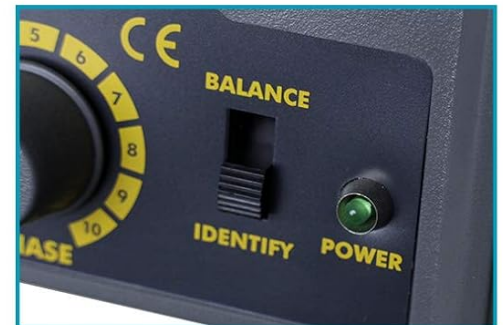
Figure 2: Control Panel of the ALLOSUN TS150. This image highlights the various controls on the detector's panel, including the amperemeter, loudspeaker, sensitivity knob, phase knob, operating mode switch, and power lamp.
