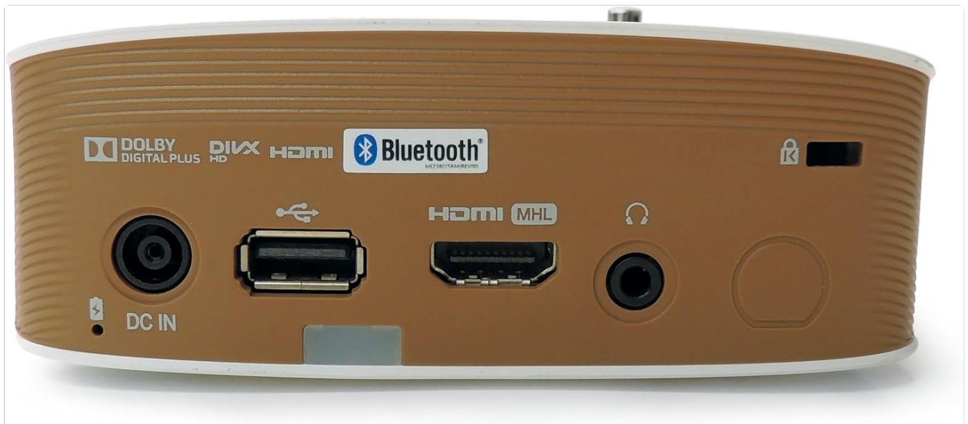
Figure 2.2: Rear panel of the Flare150, highlighting the DC IN port, USB, HDMI, and audio output connections.
