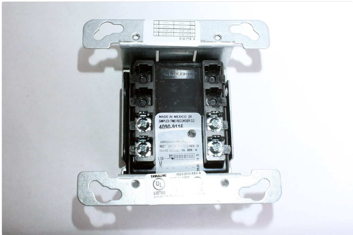
Figure 2.1: Front view of the Simplex 4090-9116 Addressable IDNet Isolator, showing terminal blocks for wiring connections.
